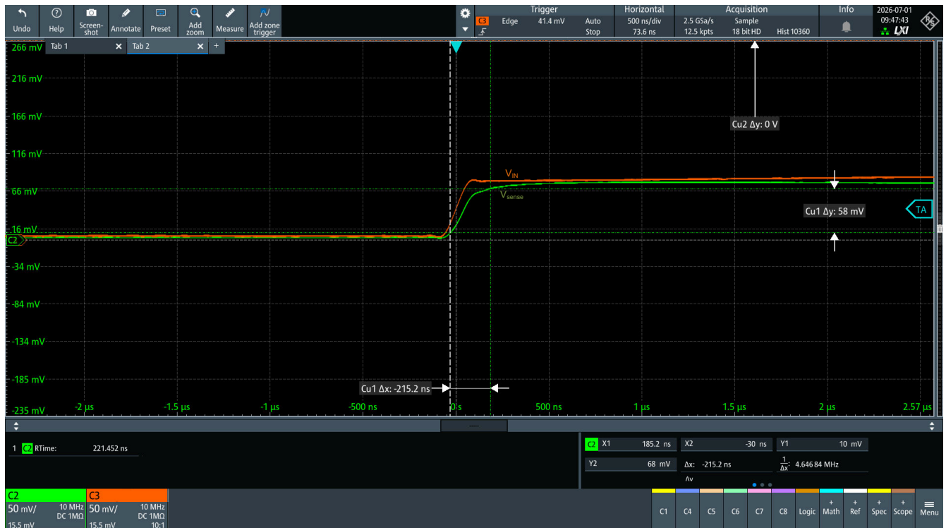
Figure 6-2. Detailed View of Transient Rise Time and Settling Behavior
