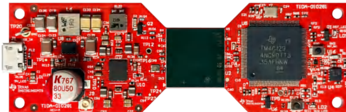
Figure 6-2. TIDA-010281 Reference Design for Safe Perception in Robotics
