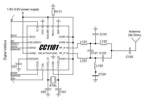
Figure 5. Schematic 868/915MHz without Single-Ended Filter
