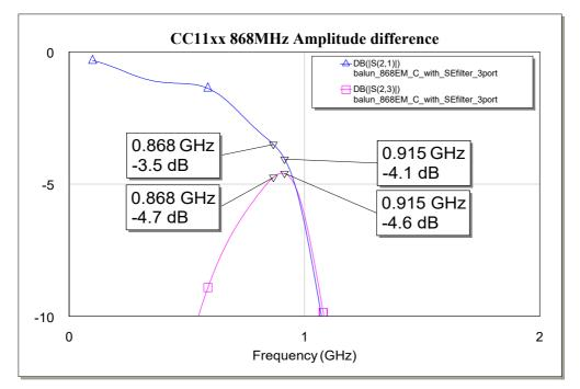
Figure 7. Amplitude Difference
