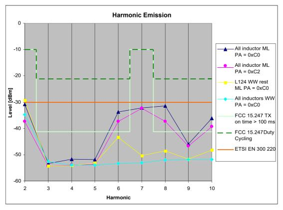
Figure 14. Conducted Harmonic Emission
