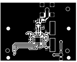
Figure 13. Layout of the Notch Filter
