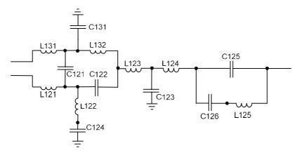
Figure 12. The Notch Filter Schematic
