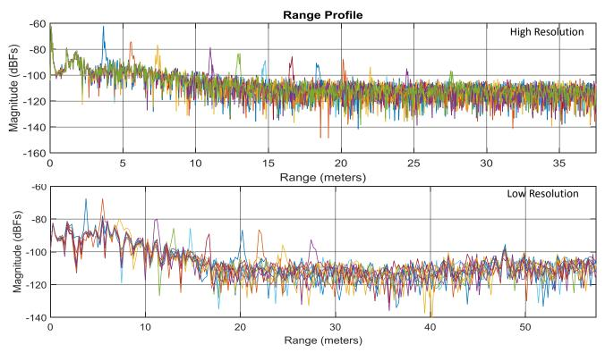
Figure 12. Range Profile of Pedestrian at Different Distances
