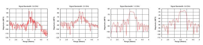
Figure 4. Range Profile of Four Bandwidth Cases With Separation of 20 cm
