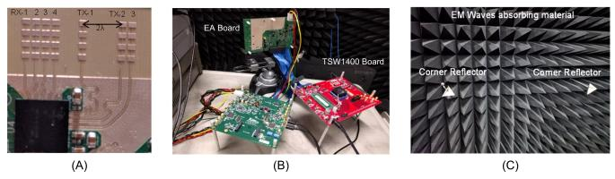
Figure 1. Etched Antennas (A); Measurement Setup (B); Anechoic Chamber With Absorbing Material (C)
