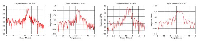
Figure 5. Range Profile of Four Bandwidth Cases With Separation of 10 cm
