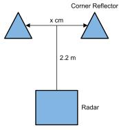
Figure 8. Experiment Setup for Angle Resolution Measurement
