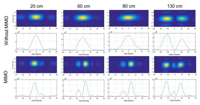
Figure 9. Range-Angle 2D Energy Plot With Different Angle Separation
