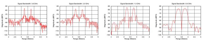
Figure 3. Range Profile of Four Bandwidth Cases With Separation of 50 cm
