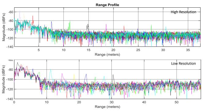
Figure 11. Range Profile of Corner Reflector (RCS = 0.1) at Different Distances
