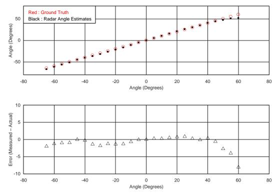
Figure 7. Angle Estimation Accuracy in Low-Resolution Mode
