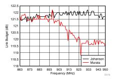
Figure 16. Sub-1 GHz Link Budget vs Frequency
