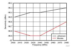
Figure 27. 2.4 GHz 1 Mbps BLE Sensitivity v Frequency
