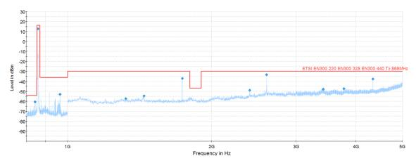
Figure 25. JTI - 868 MHz ETSI EN300 220 Radiated Emissions at Max Output Power
