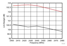
Figure 28. 2.4 GHz 1 Mbps BLE Link Budget v Frequency
