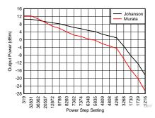
Figure 17. 868 MHz Output Power vs PA Setting
