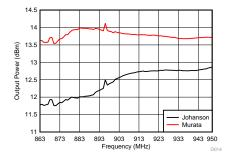
Figure 14. Sub-1 GHz Output Power vs Frequency
