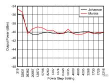
Figure 23. 868 MHz Tx 5th Harmonic vs PA Setting
