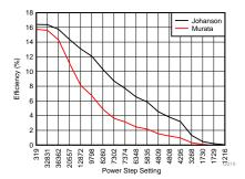
Figure 19. 868 MHz Tx Efficiency vs PA Setting
