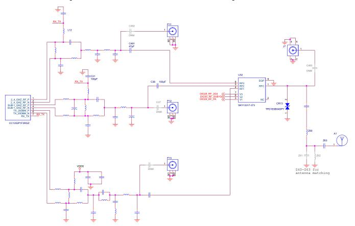
Figure 2. CC1352P LaunchPad RF Frontend Discrete Component Concept
