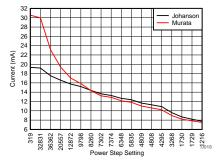
Figure 18. 868 MHz Tx Current vs PA Setting
