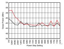
Figure 21. 868 MHz Tx 3rd Harmonic vs PA Setting
