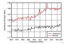
Figure 15. Sub-1 GHz Sensitivity vs Frequency
