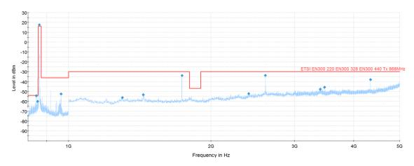
Figure 24. Murata - 868 MHz ETSI EN300 220 Radiated Emissions at Max Output Power
