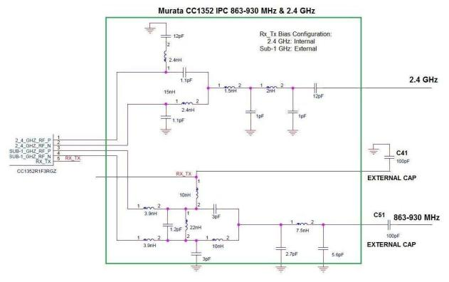
Figure 4. Murata CC1352 IPC Equivalent Circuit for 863-930 MHz & 2.4 GHz
