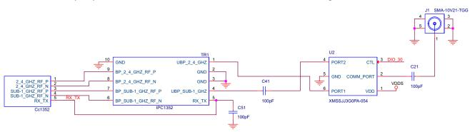
Figure 5. CC1352 IPC RF Frontend With SPDT Switch for 863-930 MHz and 2.4 GHz
