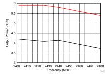
Figure 26. 2.4 GHz Output Power v Frequency
