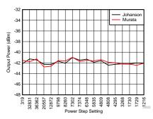
Figure 22. 868 MHz 4th Harmonic vs PA Setting
