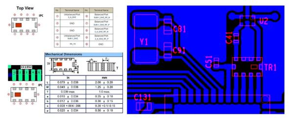
Figure 6. Component Size and Dimensions
