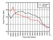
Figure 20. 868 MHz 2nd Harmonic vs PA Setting
