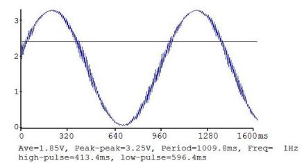
Figure 6. Example analog output of the PWM DAC.
