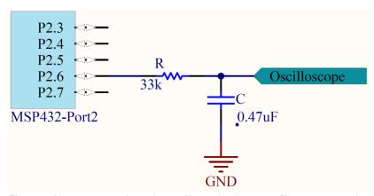
Figure 4. Use an external passive 10 Hz analog low pass filter to convert the PWM signal (P2.6 in this case) into a DAC analog output voltage.
