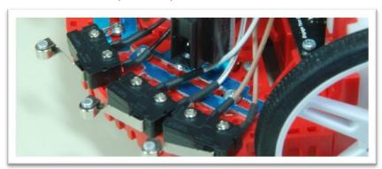
Figure 1. Bump sensors, positioned at the front of the robot.
