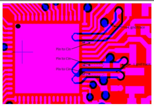
Figure 10-6. Ground Returns for Input Capacitors
