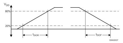
Figure 8-15. DIO Timing Diagram
