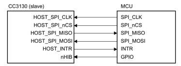
Figure 8-17. SPI Host Interface
