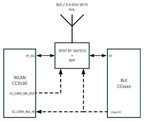
Figure 10-1. Single-Antenna Coexistence Mode Block Diagram
