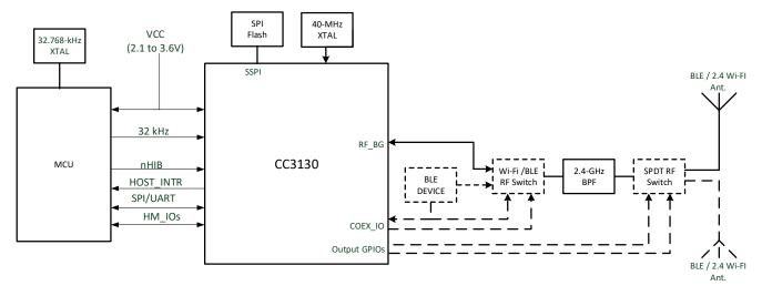
Note: The diplexer is used for the signal antenna solution. When using the antenna selection feature (dual antenna), an SPDT switch and 2 GPIO lines are required after the diplexer.
