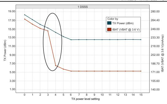
Figure 8-1. TX Power and IBAT vs TX Power Level Settings (1 DSSS)
