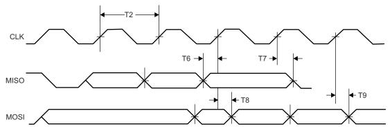
Figure 8-13. Host SPI Interface Timing
