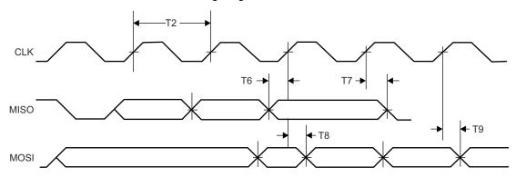
Figure 8-14. Flash SPI Interface Timing
