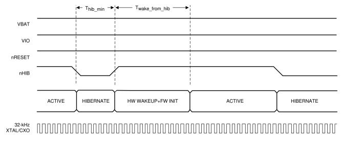
Figure 8-8. nHIB Timing Diagram
