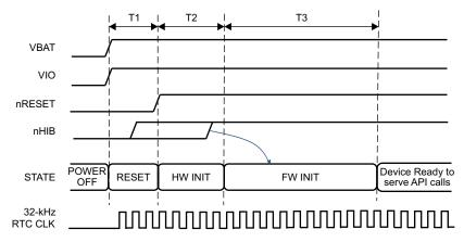
Figure 8-7. First-Time Power-Up and Reset Removal Timing Diagram (External 32-kHz Crystal)
