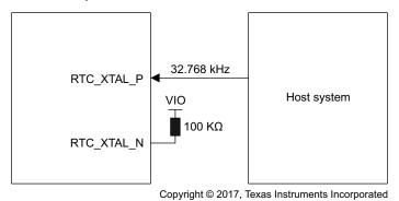
Figure 8-10. External RTC Input
