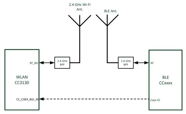
Figure 10-2. Dual-Antenna Coexistence Mode Block Diagram
