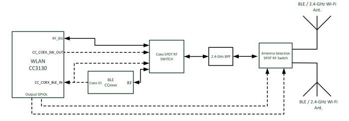
Figure 10-3. Antenna Selection Solution With Coexistence
