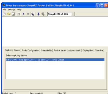
The USB dongle should be listed with chip type CC1111 and EB type CC1111 USB dongle in the "Capturing Device" tab.
