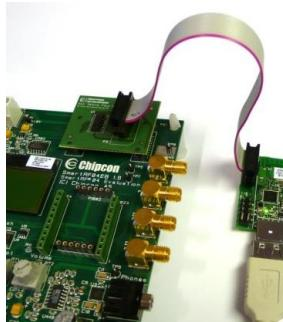
**Caution!** Avoid using other power sources for the dongle than a regular USB voltage source at max 5.5V, 500 mA.
