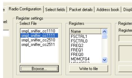
If this is the first time you use the tool, press the browse button to locate a .prs file with packet sniffer register settings for CC1111.
