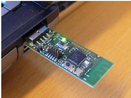
**Caution!** The CC2540 USB dongle is designed to be powered over USB, with a maximum voltage of 5.5V and maximum current of 500 mA.
