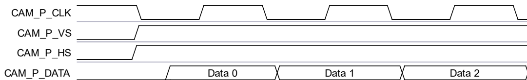
Figure 14-3. Synchronization Signals and Data Timing
