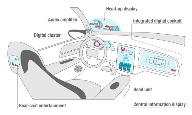
Figure 1. Components of an infotainment system.
