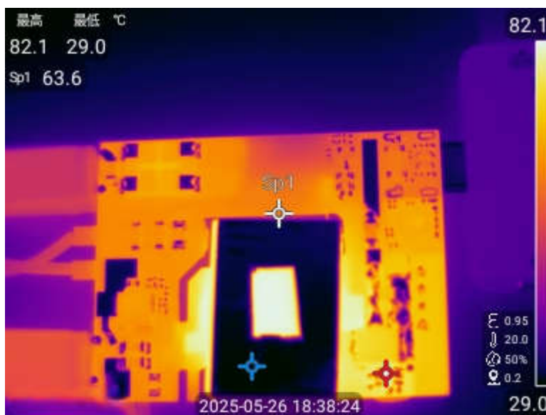
Figure 2-10. 115VAC, 20V, 2.25A
