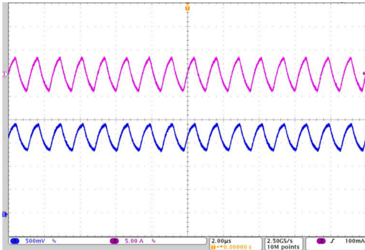
Figure 2-5. CLLC_IPRIM_TANK Signal at 800kHz
