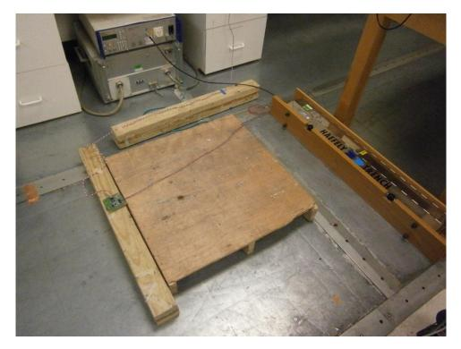
Figure B-4: EFT Test Setup
