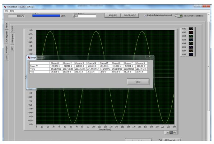
Figure 26. RMS Readings for Captured Signal
