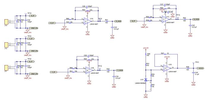
Figure 12. Earth Fault Current Signal Conditioning
