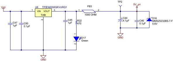
Figure 11. Primary-Side DC Output Regulator
