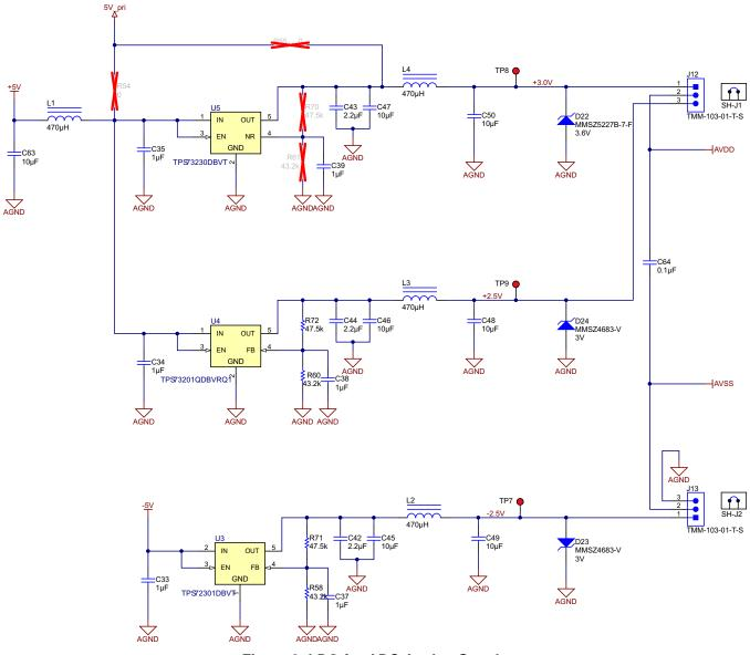
Figure 9. LDO for ADC Analog Supply
