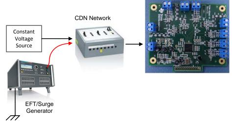
Figure 34. Surge Setup for ADC Board
