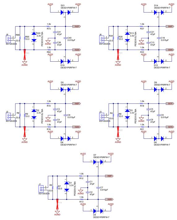
**Figure 4. Current Input Connectors**
