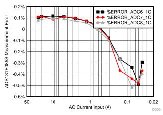
Figure 29. Input Current Vs ADC Measurement Error
