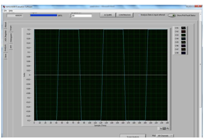
Figure 25. Waveform With Saturated Input
