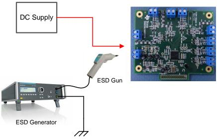
Figure 35. ESD Setup for ADC Board
