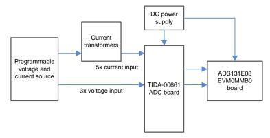
Figure 19. ADC Board Interfaced to MMB0 Board
