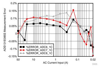
Figure 31. Input Current Vs ADC Measurement Error (2.4-V Reference)
