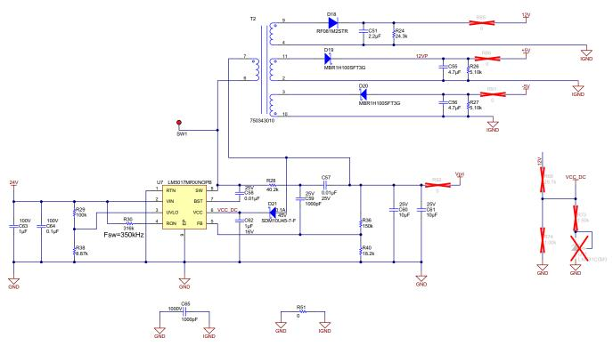
Figure 7. LM5017 Configured for Fly-Buck Operation
