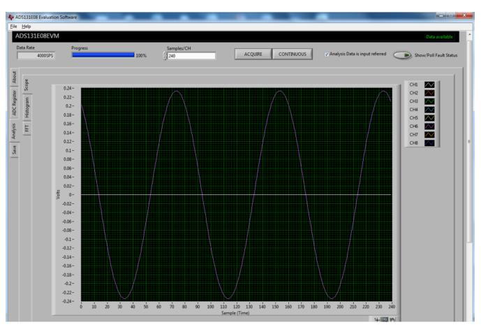
Figure 23. Waveform With 240 Samples
