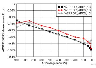
Figure 28. Input Voltage Vs ADC Measurement Error (4-V Reference)
