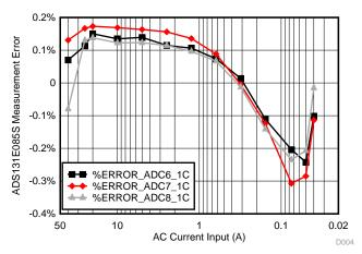
Figure 30. Input Current Vs ADC Measurement Error (4-V Reference)
