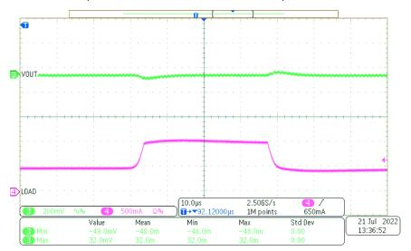
Figure 3-6. Load Transient 500-mA to 1-A with 12-Vin
