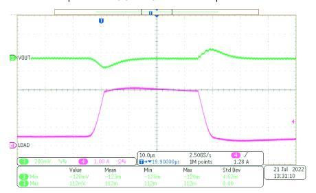
Figure 3-4. Load Transient 500-mA to 3-A with 12-Vin
