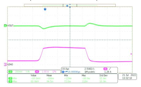
Figure 3-5. Load Transient 500-mA to 2-A with 12-Vin
