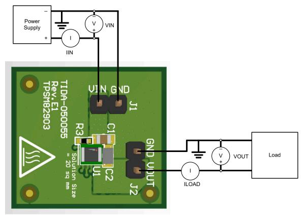
Figure 3-1. Test Setup
