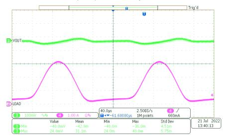
Figure 3-7. PSM to PWM Transition with 12-Vin
