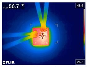
Figure 3-10. Thermal Image at Room Temperature with 12-Vin, 1.2-Vo, 2.5-A
