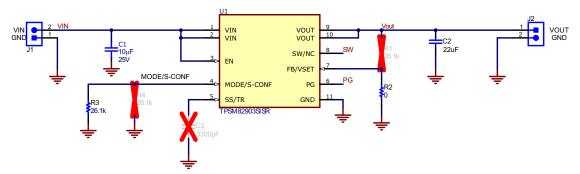
Figure 2-2. Buck Converter Circuit Design Using TPSM82903
