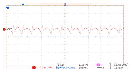
Figure 3-8. Vout Ripple at 3-A
