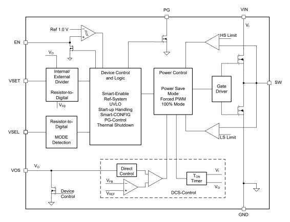
Figure 2-1. TIDA-050055 Block Diagram
