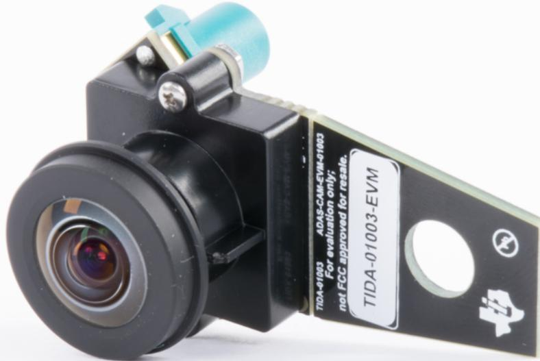
**Figure 11. TIDA-01003 Completed Assembly**
