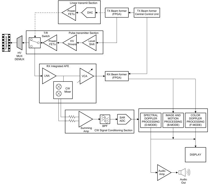
Figure 1 shows the block diagram of an ultrasound imaging system.
