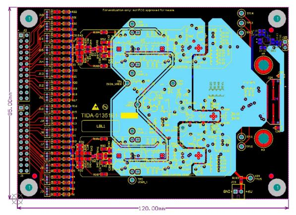
Figure 31. TIDA-01351 Power Supply Layout Recommendations
