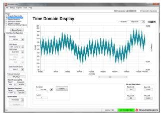
Figure 15. ADC Sensitivity Measured With 10-µVp-p Input Signal at 2 kHz
