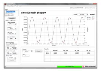
Figure 22. Time Domain Display of I and Q signals at 2 kHz
