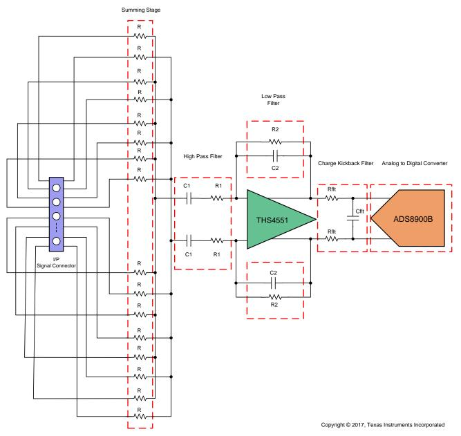
Figure 3. Summing Stage, Active Filter, ADC Driver, and Charge Kickback Filter Circuit
