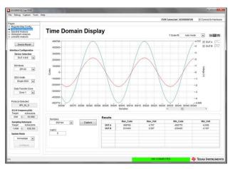
Figure 24. Time Domain Display of I and Q Signals at 20 kHz (One Channel is Given Half of the Gain Compared to the Other Channel)
