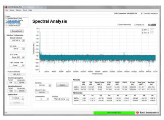
Figure 26. ADC AC Performance With a Gain of 10 at 2 kHz Using 18-Bit ADS8910B
