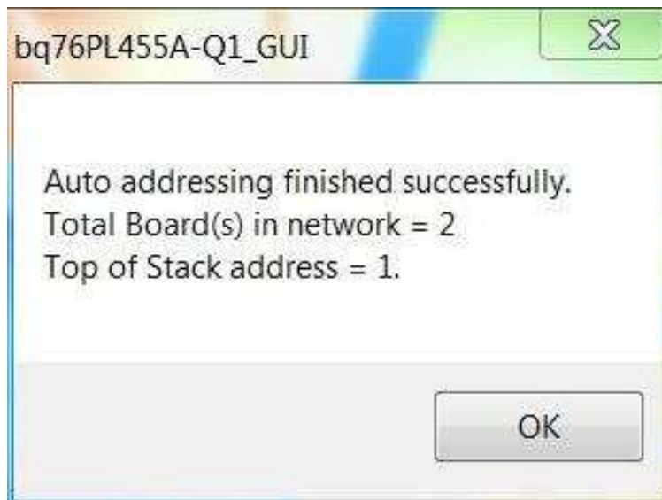
Figure 3. bq76PL455A GUI Detecting Two Board Stack
