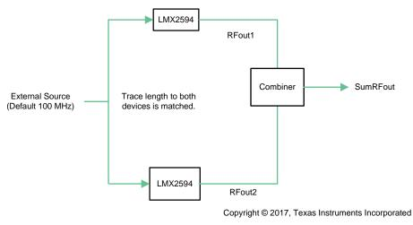
Figure 1. Block Diagram
