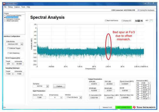
Figure 23. Spectral Analysis Before Internal Offset Calibration
