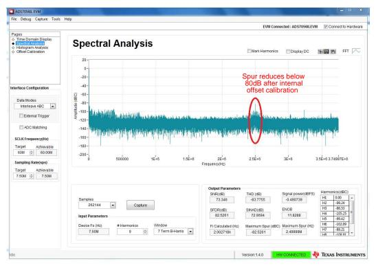
Figure 24. Spectral Analysis After Internal Offset Calibration
