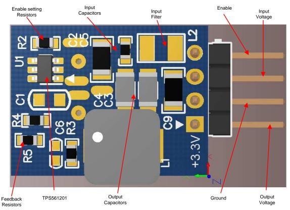
Figure 4. TIDA-01447 PCB With Functional Blocks
