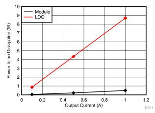
Figure 3. Comparison of Power Dissipated
