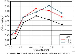
Figure 10. Line and Load Regulation at -30°C
