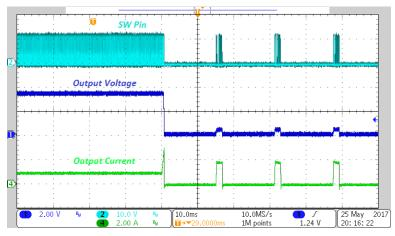
**Figure 18. Overcurrent Protection**
