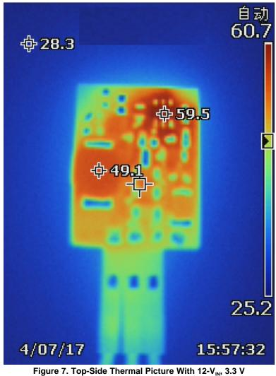
gure 7. Top-Side Thermal Picture With 12-V<sub>IN</sub>, 3.3 at 1-A Output
