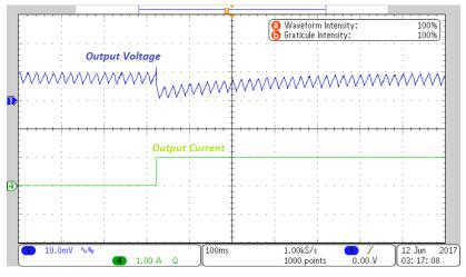
Figure 14. Transient Response From 10-mA to 1-A Output Load
