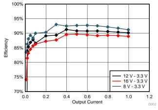
Figure 6. TIDA-01447 Efficiency
