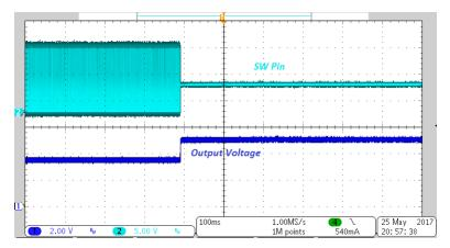
Figure 20. Overvoltage Protection From 5 to 6 V
