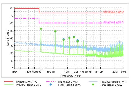
Figure 22. Conducted Emission Test Result
