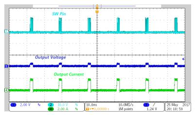
Figure 19. Short-Circuit Protection
