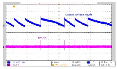
Figure 13. Output Voltage Ripple at No Load Output
