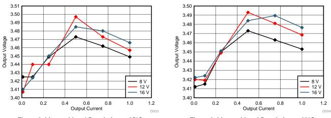
Figure 8. Line and Load Regulation at 85°C
