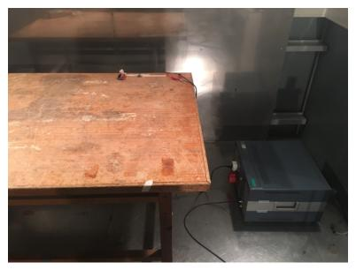
Figure 21. Conducted Emission Test Setup
