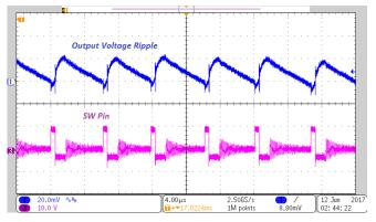
Figure 12. Output Voltage Ripple at 10-mA Output Load
