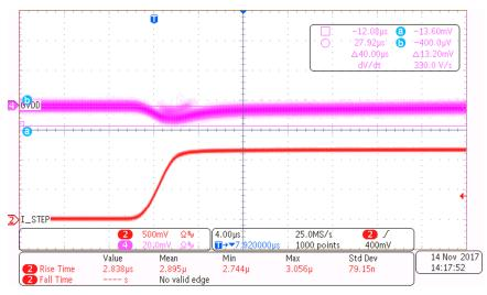
Figure 17. GVDD Rail—30-A to 50-A Transient Undershoot, 10% Duty Cycle
