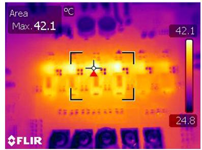
Figure 26. Dual-Rail Power Stage Temperatures
