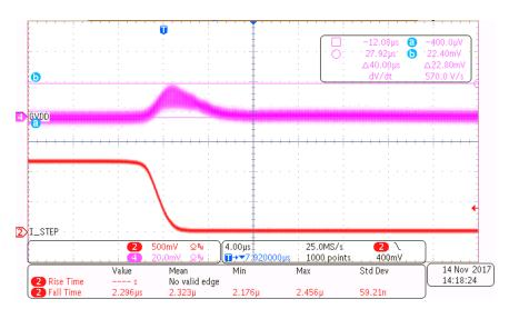
Figure 18. GVDD Rail—30-A to 50-A Transient Overshoot, 10% Duty Cycle
