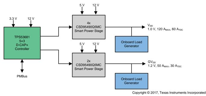
Figure 1. Block Diagram
