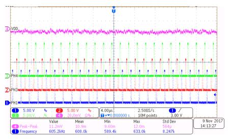
Figure 9. VDD Rail—Steady State, 120 A
