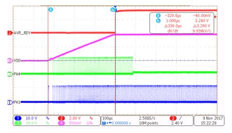
Figure 27. VDD Rail—10-A Start-up
