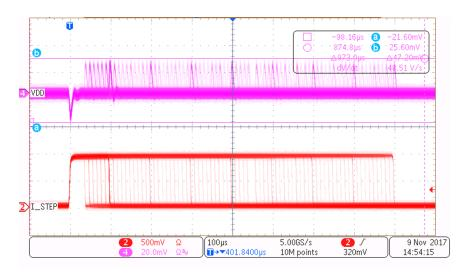
Figure 16. VDD Rail-60-A to 120-A Transient, 10% to 80% Duty Cycle Sweep
