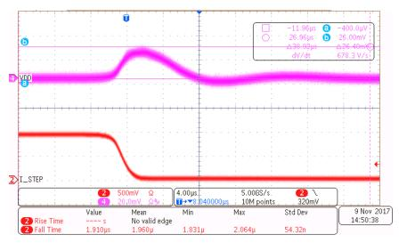
Figure 15. VDD Rail—60-A to 120-A Transient Overshoot, 10% Duty Cycle
