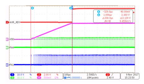
Figure 28. VDD Rail—60-A Start-up
