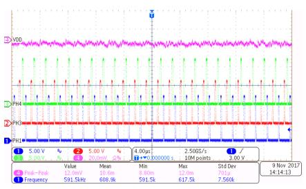
Figure 8. VDD Rail—Steady State, 60 A
