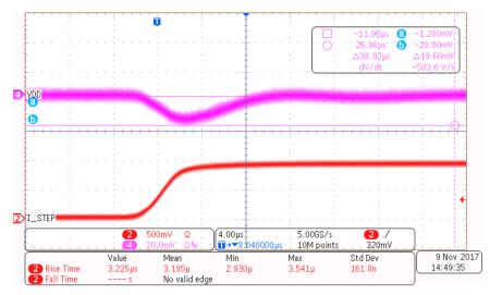
Figure 14. VDD Rail—60-A to 120-A Transient Undershoot, 10% Duty Cycle
