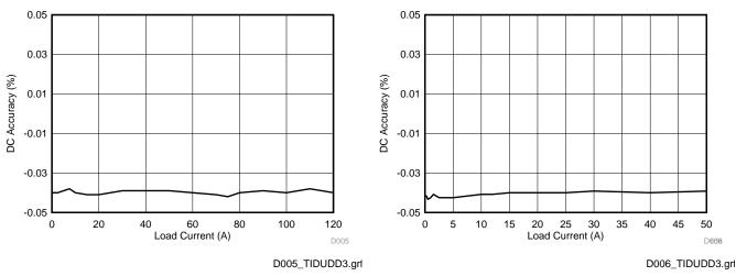
Figure 12. VDD Rail DC Accuracy
