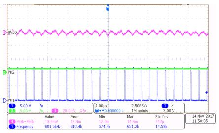
Figure 10. GVDD Rail—Steady State, 10 A
