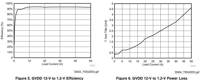
Figure 6. GVDD 12-V to 1.2-V Power Loss
