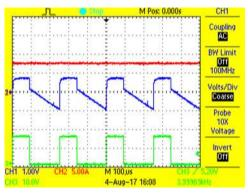
Figure 59. 8-A DC Current in Phase U AC Coupled
