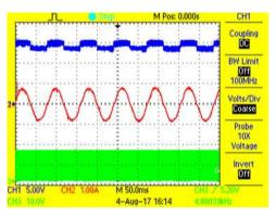
Figure 60. Sinusoidal Current in Phase U
