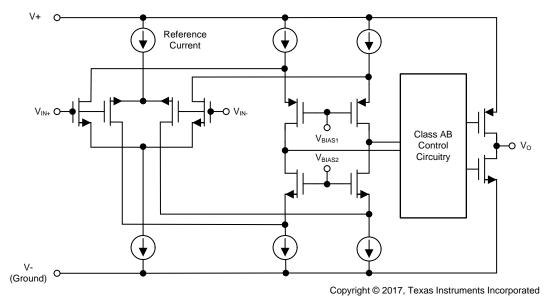
Figure 6. Functional Block Diagram of TLV9062
