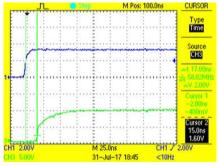
Figure 39. Low-Side Phase W Turnon Propagation Delay (17 ns)
