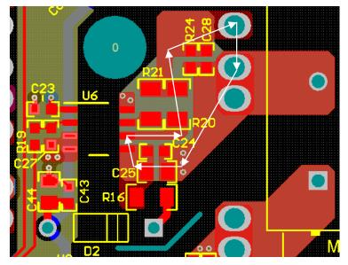
Figure 73. High-Side Gate Turnon Loop
