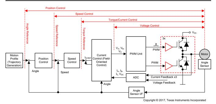
Figure 1. Generic Motor Control Block
