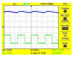
Figure 50. 50% Duty Cycle DC Coupled
