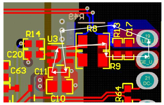
Figure 71. Low-Side Gate Driver Turnon Loop
