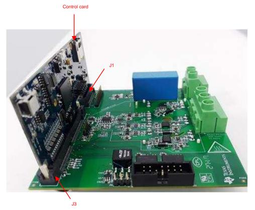
Figure 30. Control Card Connection to TIDA-01456
