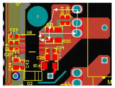
Figure 74. High-Side Gate Turnoff Loop
