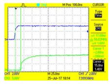
Figure 37. Low-Side Phase U Turnon Propagation Delay (17 ns)
