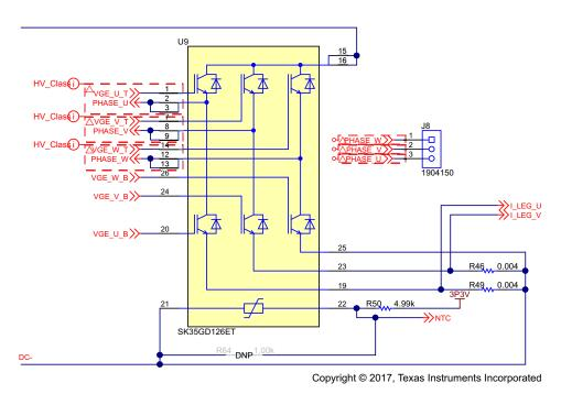
Figure 15. Three-Phase Inverter Stage
