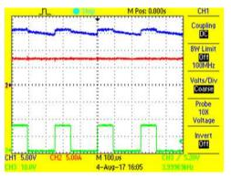
Figure 58. 8-A DC Current in Phase U DC Coupled
