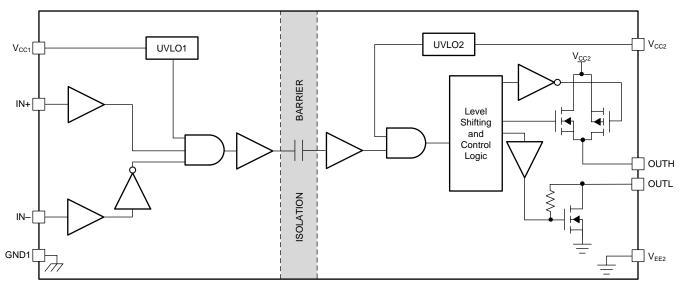
Figure 4. Functional Block Diagram of UCC5320S
