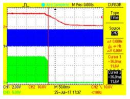
Figure 33. High-Side Gate Driver (UCC5320S) UVLO Turnoff
