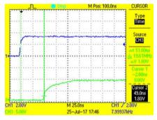
Figure 44. High-Side Phase U Turnon Propagation Delay (51 ns)
