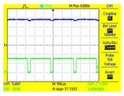
Figure 54. 90% Duty Cycle DC Coupled
