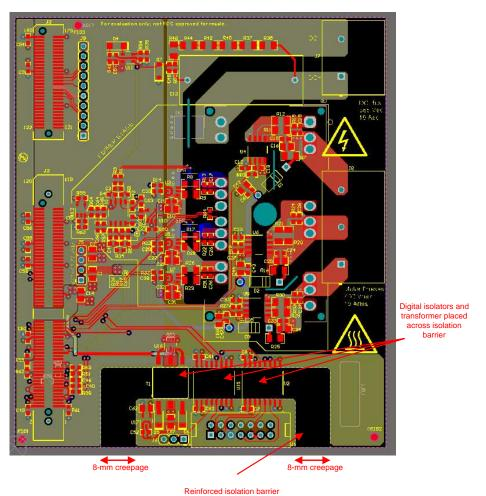
Figure 70. Reinforced Isolation Barrier and Creepage Spacing
