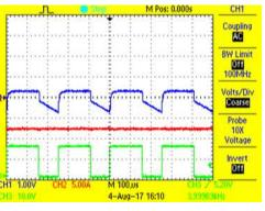
Figure 57. –8-A DC Current in Phase U AC Coupled
