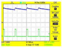
Figure 52. 10% Duty Cycle DC Coupled
