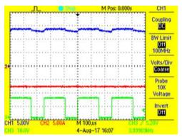
Figure 56. –8-A DC Current in Phase U DC Coupled
