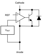
Figure 7. Functional Block Diagram of TLV431
