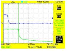
Figure 47. High-Side Phase U Turnoff Propagation Delay (51 ns)
