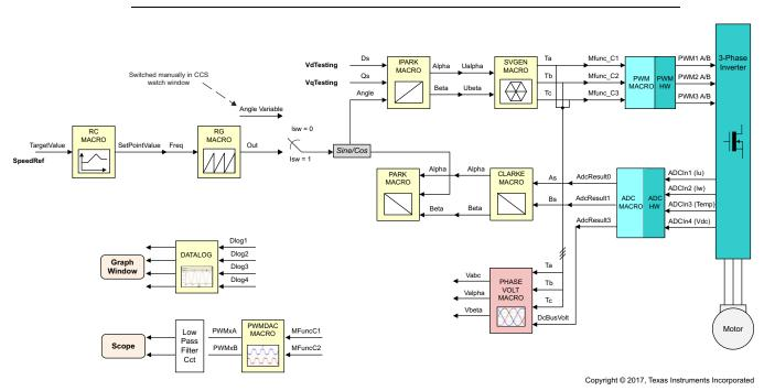
Figure 31. PWM Control Software
