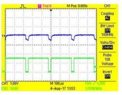
Figure 55. 90% Duty Cycle AC Coupled
