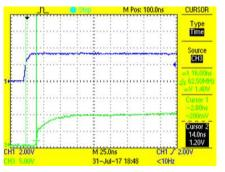
Figure 38. Low-Side Phase V Turnon Propagation Delay (16 ns)
