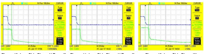
Figure 40. Low-Side Phase U Turnoff Propagation Delay (17 ns)
