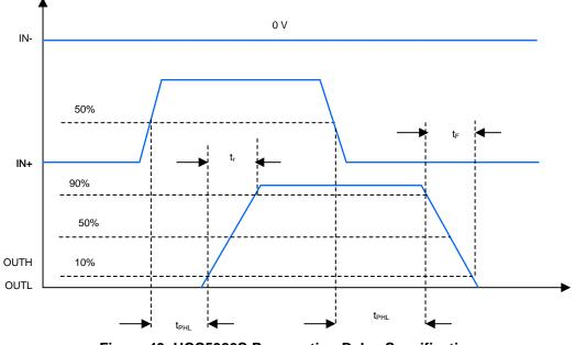
Figure 43. UCC5320S Propagation Delay Specification
