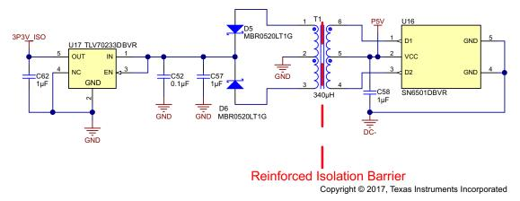
Figure 25. Isolated 3.3-V Power Supply Generation
