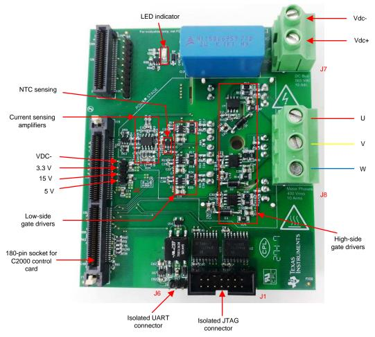
Figure 26. Top View of TIDA-01456 PCB
