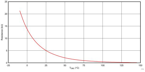
Figure 21. NTC Characteristics
