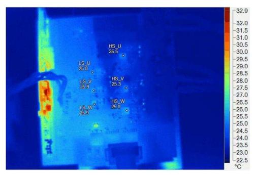
Figure 69. Measurement of Operational Temperature Rise of Gate Drivers
