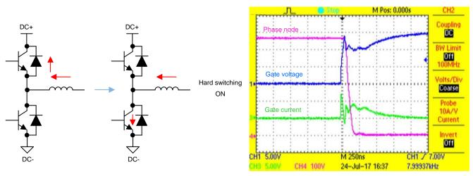
Figure 61. Hard Switch Turnon (Low Side)
