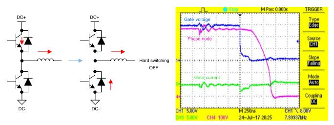
Figure 66. Hard Switch Turnoff (High Side)
