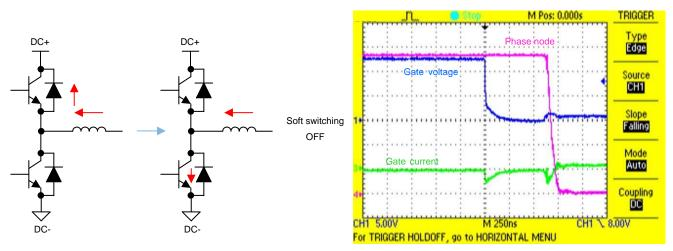
Figure 68. Soft Switch Turnoff (High Side)
