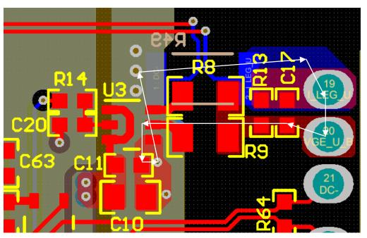
Figure 72. Low-Side Gate Driver Turnoff Loop
