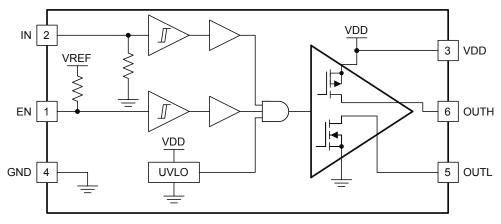
Figure 5. Functional Block Diagram of UCC27531
