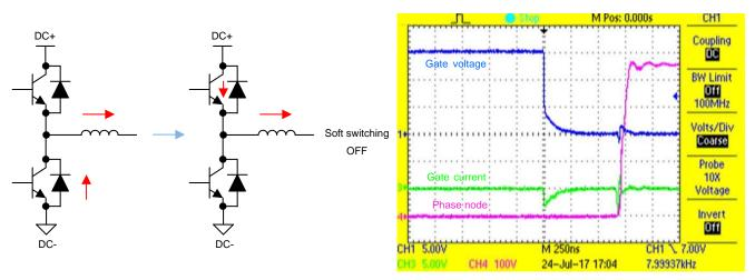
Figure 64. Soft Switch Turnoff (Low Side)
