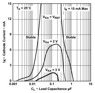
Figure 20. TLV431 Stability Boundary Condition
