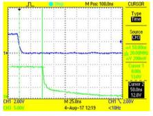
Figure 49. High-Side Phase W Propagation Delay (50 ns)
