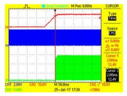
Figure 34. High-Side Gate Driver (UCC5320S) UVLO Turnon
