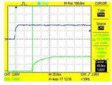
Figure 46. High-Side Phase W Turnon Propagation Delay (52 ns)
