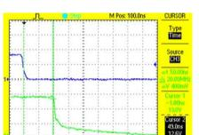
Figure 48. High-Side Phase V Turnoff Propagation Delay (50 ns)
