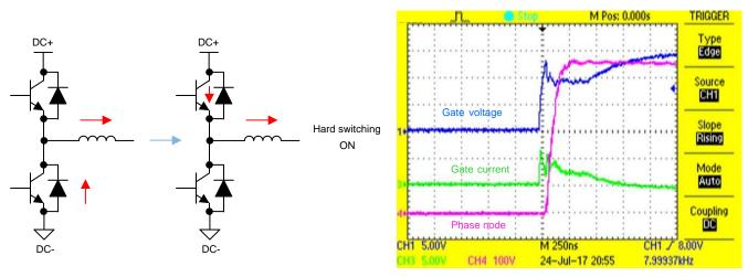
Figure 65. Hard Switch Turnon (High Side)
