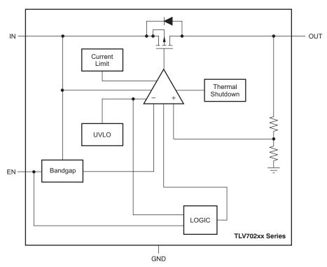
Figure 10. Functional Block Diagram of TLV702
