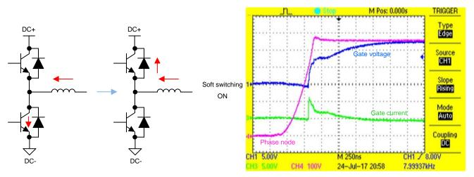
Figure 67. Soft Switch Turnon (High Side)
