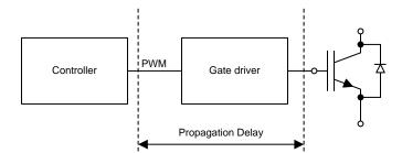
Figure 35. PWM Propagation Delay
