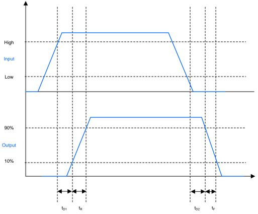
Figure 36. UCC27531 Propagation Delay Specification
