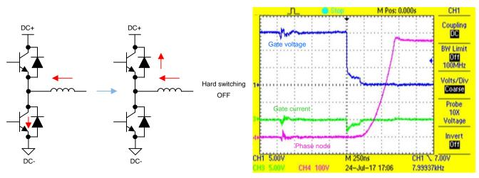
Figure 62. Hard Switch Turnoff (Low Side)
