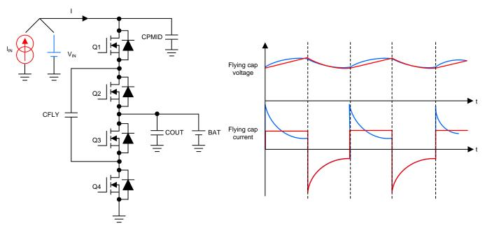
Figure 5. Switching Waveforms Difference With Current versus Voltage Source
