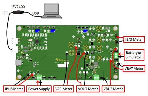
Figure 10. PWR881 Test Connections
