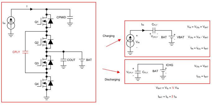
Figure 3. Simplified Switched Cap Circuit (Single Phase)
