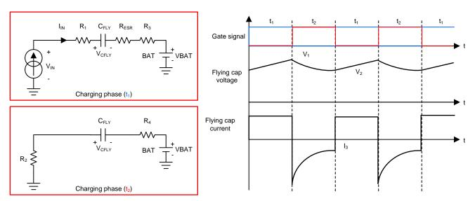
Figure 4. Switching Waveforms With Current Source
