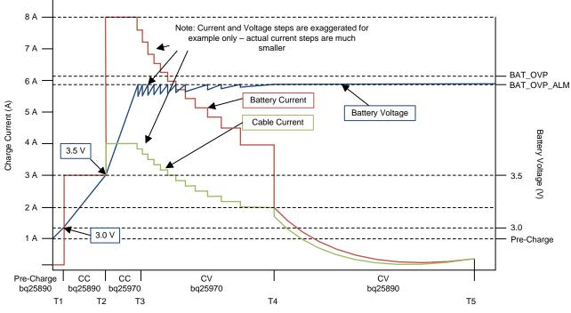
Figure 2. Ideal Charge Cycle Operation
