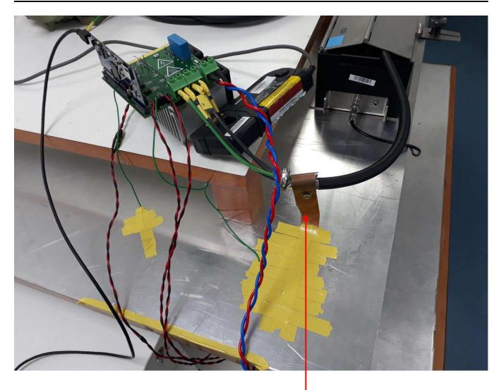
Copper strap connection from cable shield to table reference
