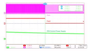
Figure 53. Fault Signal Detection
