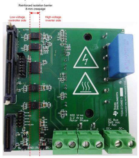
Figure 21. High-Voltage Inverter Side, Control Side, and Reinforced Isolation Barrier
