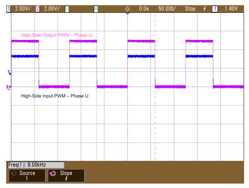
Figure 27. Input and Output PWM Waveforms of ISO7760F
