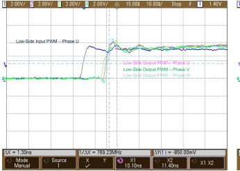
Figure 34. Low-Side PWM Propagation Delay Skew—Rising Edge (Measured 1.3 ns)
