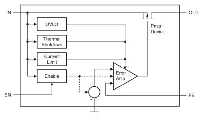
Figure 7. Functional Block Diagram of TPS7A4201
