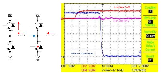
Figure 41. Hard Switch on—Low-Side IGBT Captured at -5-A Motor Current
