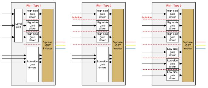
Figure 1. IPM Types—PWM Input Perspective
