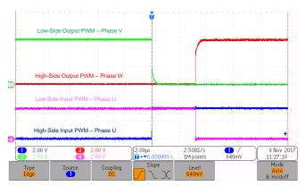
Figure 45. Rising Edge of PWM Signal Interlock (Phase U)
