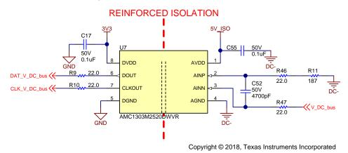
Figure 13. Schematic of DC Bus Voltage Sensing Using AMC1303M2520
