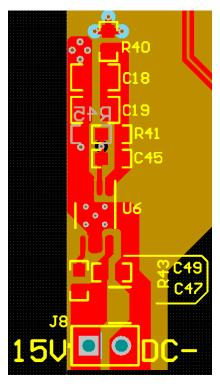
Figure 62. Layout for TPS7A4201
