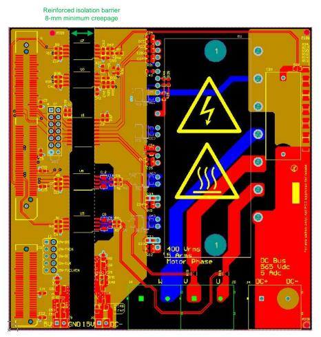
Figure 57. Reinforced Isolation Barrier and Creepage Spacing
