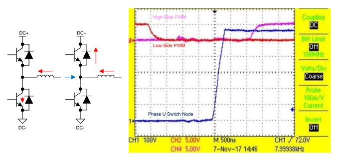
Figure 40. Soft Switch on—High-Side IGBT Captured at –5-A Motor Current
