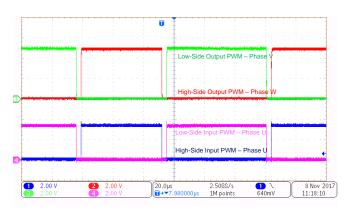
Figure 43. Normal Operation of High-Side and Low-Side PWM Signals (Phase U)
