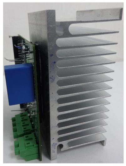
Figure 23. IPM Interface to Heat Sink
