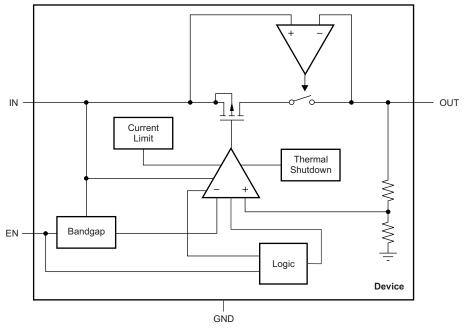
Figure 8. Functional Block Diagram of TPS706
