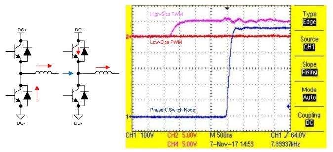
Figure 39. Hard Switch on—High-Side IGBT Captured at 5-A Motor Current
