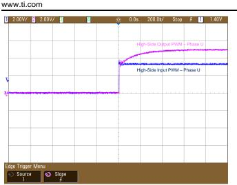
Figure 28. Rising Edge of PWM Signal— Propagation Delay Hardware, Software, Testing Requirements, and Test Results
