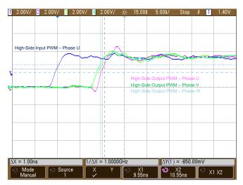
Figure 32. High-Side PWM Propagation Delay Skew—Rising Edge (Measured 1 ns)
