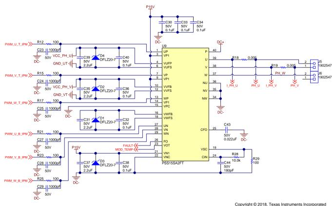
Figure 9. Schematic of Three-Phase Inverter Using IPM
