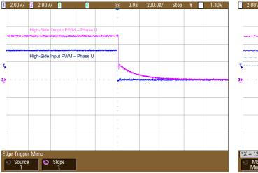
Figure 30. Falling Edge of PWM Signal— Propagation Delay
