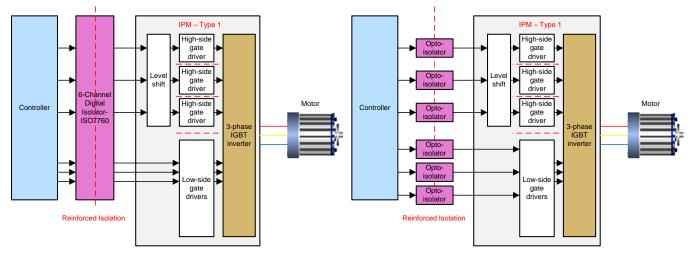
Figure 2. Using Six-Channel Digital Isolator
