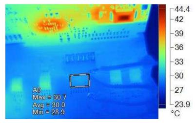
Figure 38. ISO7760F Temperature Rise After 30 Minutes
