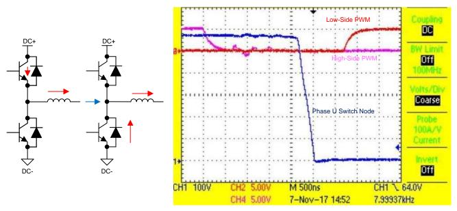
Figure 42. Soft Switch on—Low-Side IGBT Captured at 5-A Motor Current
