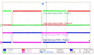
Figure 44. Negative Dead Time Fault Purposefully Introduced to Check Interlocking Function (Phase U)
