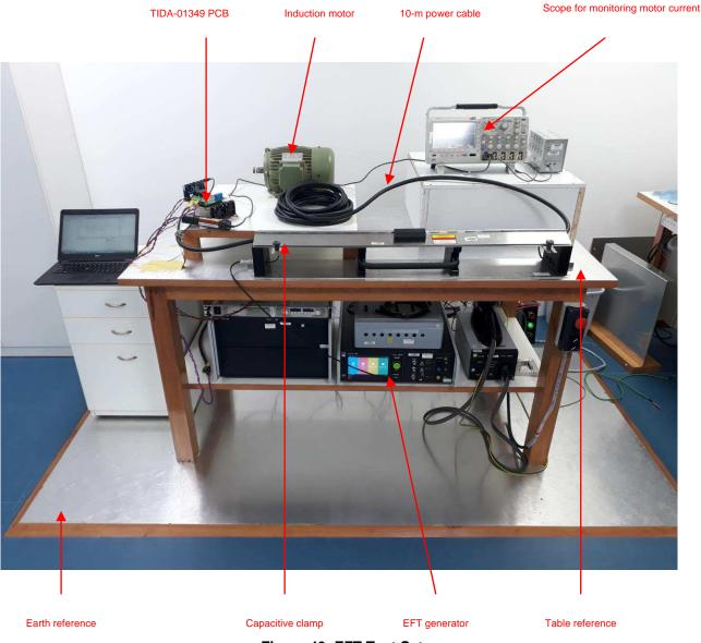
Figure 49. EFT Test Setup
