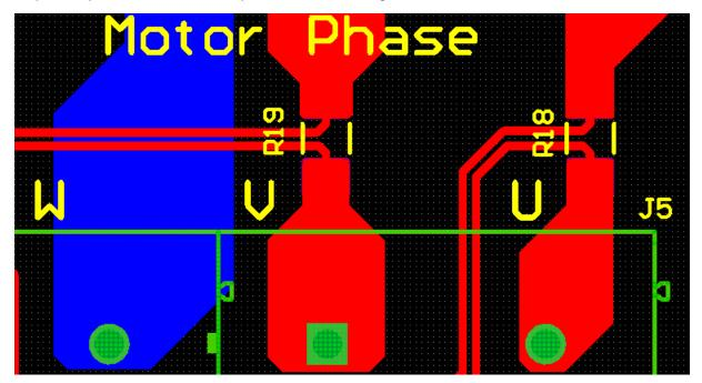
Figure 58. Kelvin Connection to Shunt Resistors
