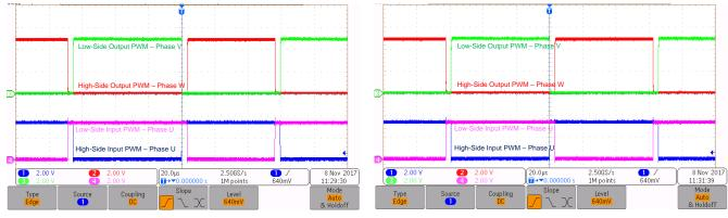
Figure 47. Interlocking (Phase V)
