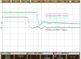
Figure 35. Low-Side PWM Propagation Delay Skew—Falling Edge (Measured 1.2 ns)
