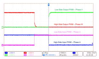
Figure 46. Falling Edge of PWM Signal Interlock (Phase U)
