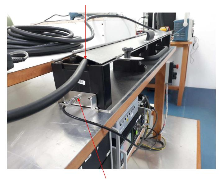
BNC connector to apply EFT burst from generator to capacitive clamp. Should be on inverter side
