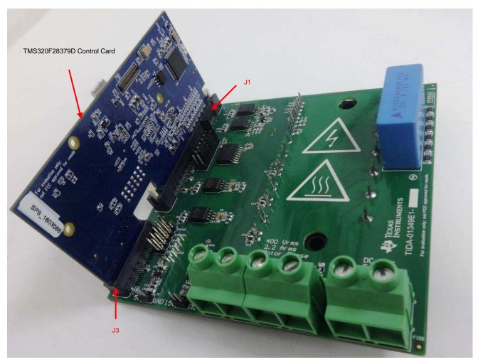
Figure 24. Control Card Connection to TIDA-01349
