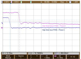
Figure 31. Falling Edge of PWM Signal Zoomed (Measured 12.7 ns)
