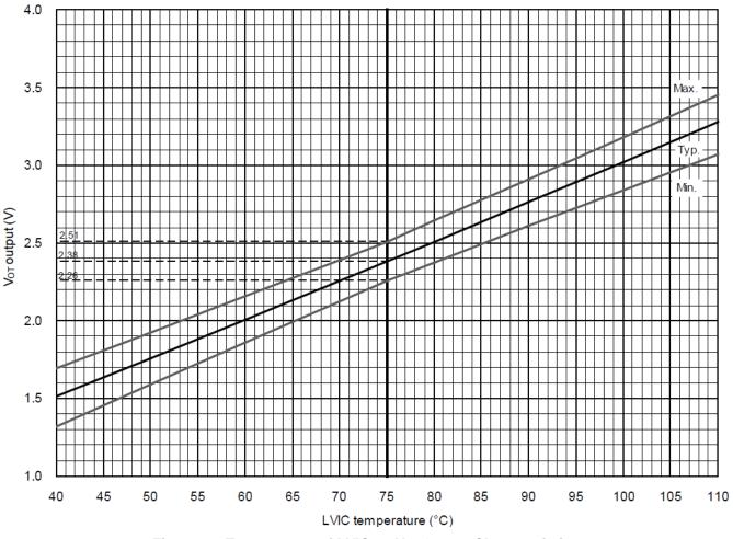
Figure 16. Temperature of LVIC vs V<sub>ot</sub> Output Characteristics
