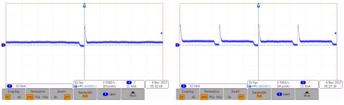
Figure 36. Icc2 at 2-kHz PWM
