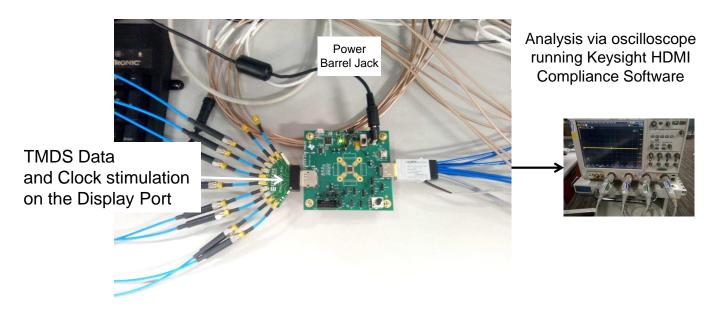
Figure 15. HDMI Test Setup for DP159
