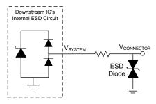
Figure 9. Low Clamping ESD Protection
