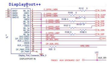
Figure 12. HDMI or DP++ Input Connector
