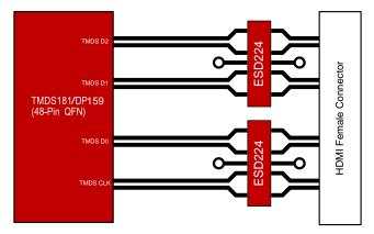
Figure 10. ESD224 Protection Schematic
