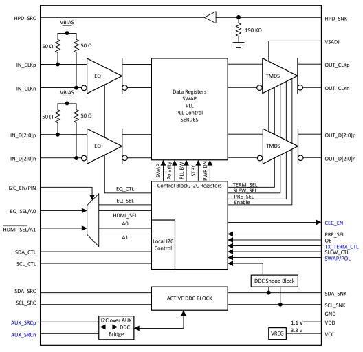
Figure 4. SN65DP159 Functional Block Diagram
