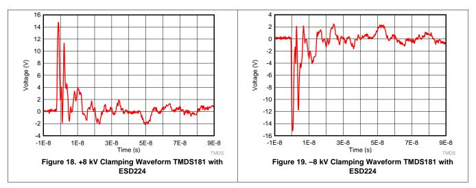
The clamping voltage at 30 ns as can be seen in the waveform is much lower than the required voltage shown in Figure 5. The board was then struck 10 times per the IEC61000-4-2 standard at one second intervals with  $\pm 12$  kV ESD to show the full protection of the ESD224. Afterwards it was ran back through the HDMI compliance shown in Table 3.
