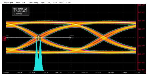
Figure 24. ±12 kV DP158 with ESD224 and CMC Post-test Eye Diagram
