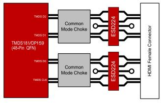
Figure 11. ESD224 and CMC Protection Schematic
