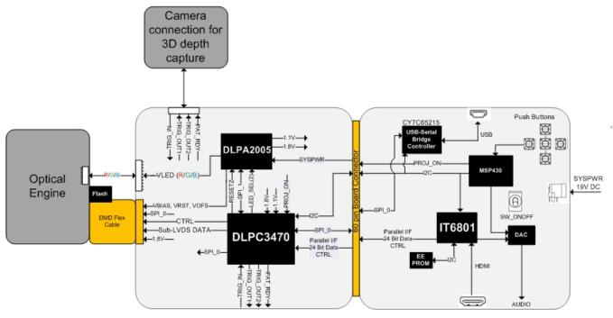
Figure 3. TIDA-080001 Block Diagram
