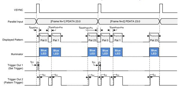
Figure 13. Internal Pattern Streaming Timing Diagram
