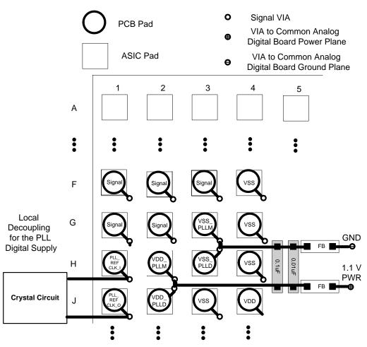
Figure 17. PLL Filter Layout
