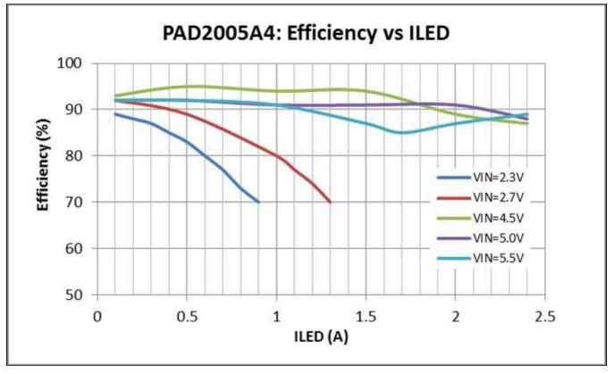
Figure 20. Measured Typical Power Converter Efficiency as a Function of ILED for Several Supply Voltages (V<sub>OUTmax</sub> = 4.8 V for Each Supply)
