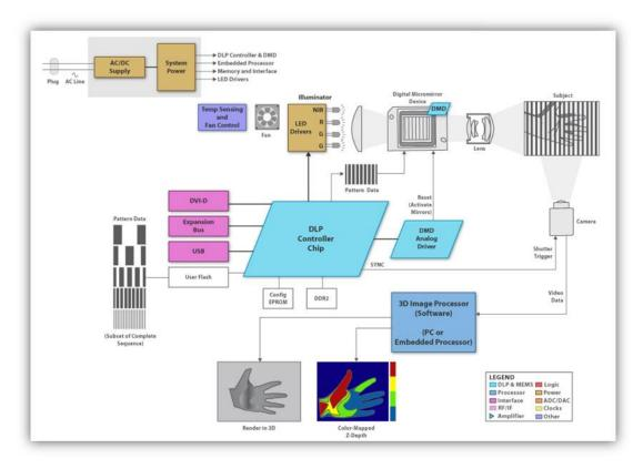
Figure 1. 3D Scanner System Block Diagram
