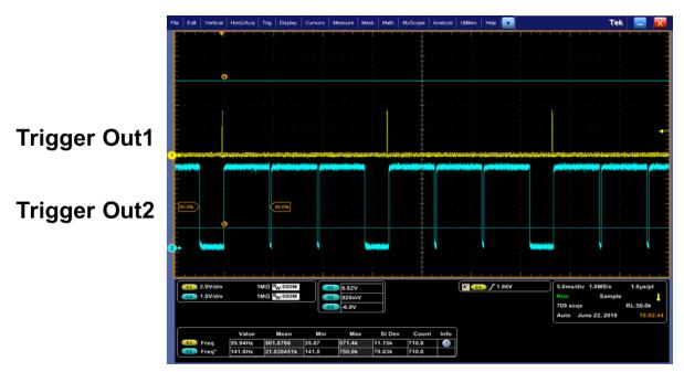
Figure 14. Scope Plots of Trigger Out1 and Trigger Out2 (24-bit Monochrome)
