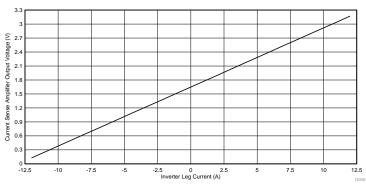
Figure 32. Inverter Leg Current vs Output Voltage Transfer Function Op Amp
