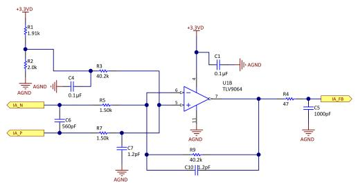
Figure 9. Inverter Leg Sensing Circuit for Two- or Three-Shunt FOC
