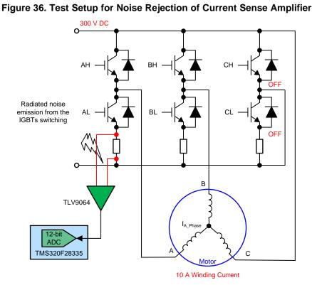
The DC bus voltage is set at 300 V, and the winding current is at 10 A. PWM is applied to Phase A and Phase B. Phase C is left open. Figure 37 shows the PWM signals, the PWM signal driving the high-side IGBT for Phase A has 10% duty, and the low-side IGBT is kept off. The PWM signal driving high-side IGBT for Phase B has 2.5% duty, and the frequency is set at 15 kHz.
