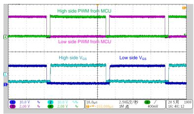
Figure 19. Low-Side and High-Side Gate Driver Voltage from UCC27712
