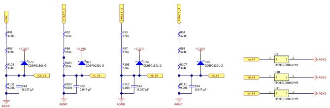
In Figure 13, PHASE\_A, PHASE\_B, and PHASE\_C are the phase voltages. These voltages are properly scaled and fed to the MCU through VA\_FB, VB\_FB, and VC\_FB. The maximum phase voltage feedback measurable by the MCU can be calculated as Equation 16 shows, considering the maximum voltage for the ADC input is 3.3 V.
