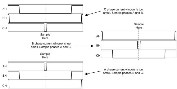
Figure 2. Using Three-Shunt Current Sampling Technique
