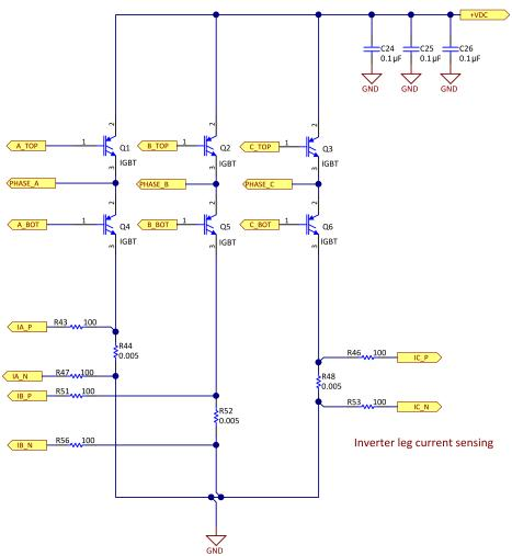
Figure 7. Three-Phase Inverter With Shunt Resistors
