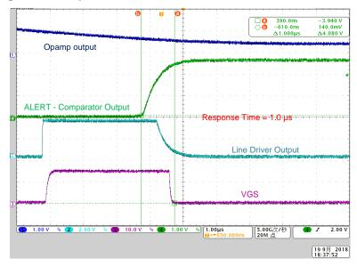
The response time of the overcurrent detection is less than 1.0 µs in hardware protection, which is fast enough to protect an IGBT (IGBTs typically have more than a 5-µs short-circuit capability). The lowest propagation delay of gate driver and line driver enables the fast turnoff of the IGBTs during an overcurrent event.
