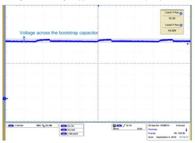
Figure 24. Voltage Ripple Across Bootstrap Capacitor
