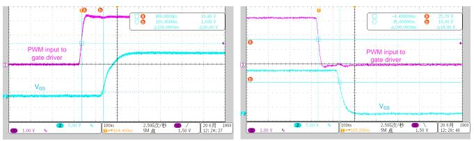
Figure 25. Gate Driver Propagation Delay During PWM Turnon and Turnoff
