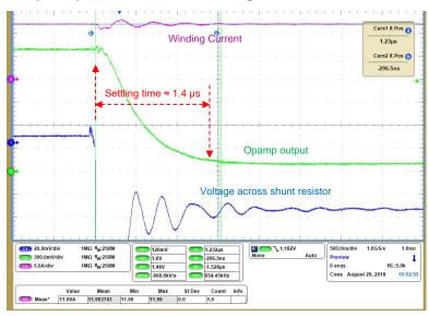
Figure 30. Step Response of Current Sensing Circuit With 12-A Positive Current
