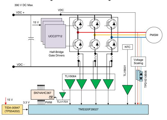
Figure 5. TIDA-010023 Block Diagram
