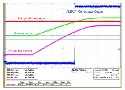
Figure 43. Overcurrent Detection for Positive Current at 1.0 ms/div
