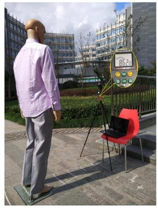
For the high ambient light operation, only model B is chosen for the test. Comparing with the same position of Scene 1, sensor performance under sunlight operation can be observed and effects of high ambient light can be concluded. In Figure 50, the red line shows the test results comparing with gray line which is sensor performance in Scene 1.
