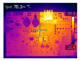
Figure 9. Thermal Characteristics for 40 V<sub>in</sub>
