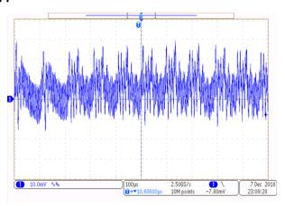
Figure 10. Output Voltage Ripple 20 V<sub>in</sub>
