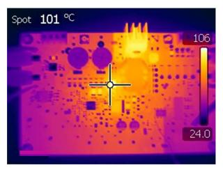
Figure 8. Thermal Characteristics for 20  $V_{\rm in}$
