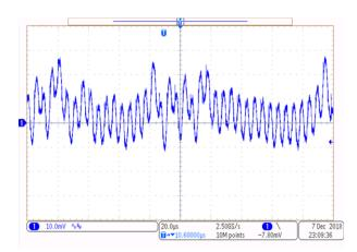
Figure 11. Output Voltage Ripple 20 V<sub>in</sub> With Smaller Time Scale
