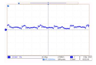
Figure 14. Output Voltage Ripple of TPS50601A-SP EVM Supplied From UC1843A-SP
