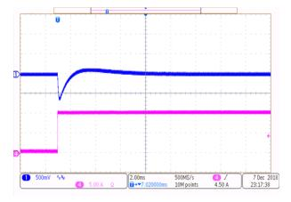
Figure 17. Partial Load Step Up With 20 V<sub>in</sub>
