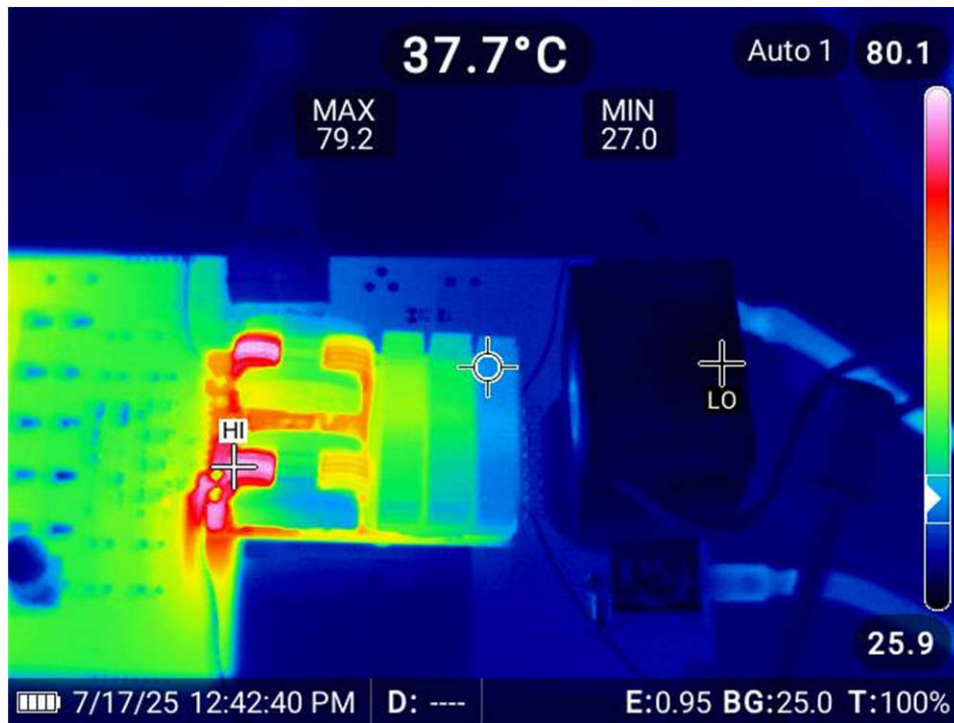
Figure 3-6. Thermal Capture (48V–12V, 2kW, 25°C Ambient, 41.2 Cubic Feet per Minute Airflow)
