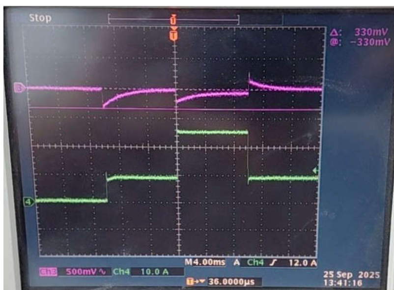
Figure 3-7. Transient Response for 48V Input Voltage with 25% to 75% To 25% Load Changes with 5A/us
