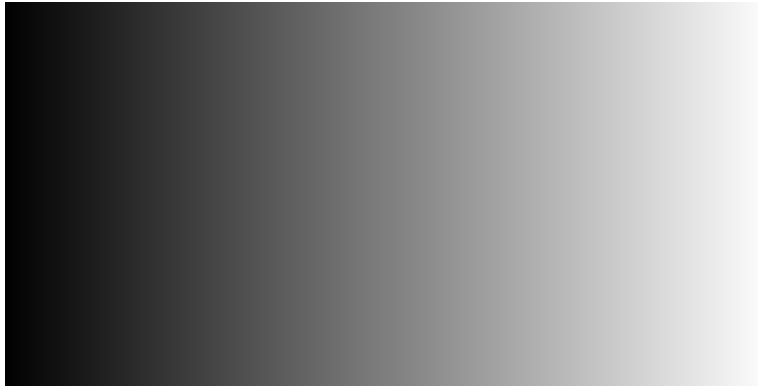
Figure 5-8. Test Pattern - Horizontal Ramp
