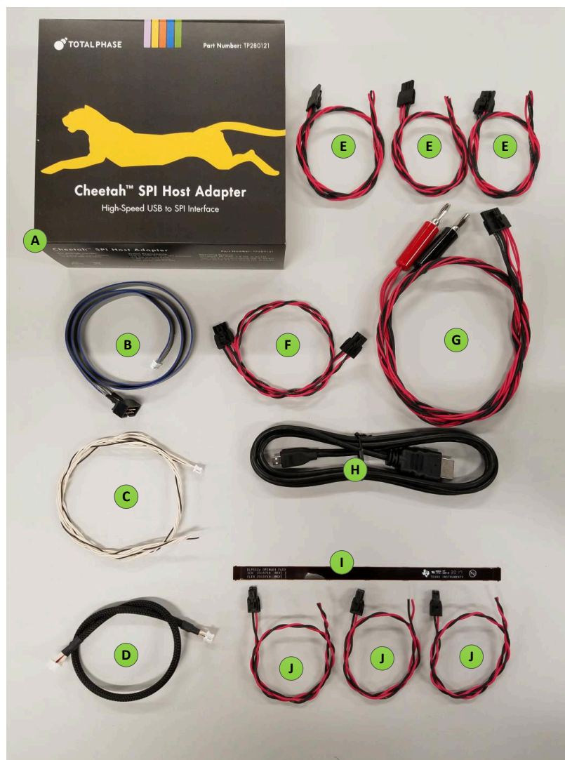
Figure 1-3. Cables Included in DLP5531-Q1 Electronics EVM
