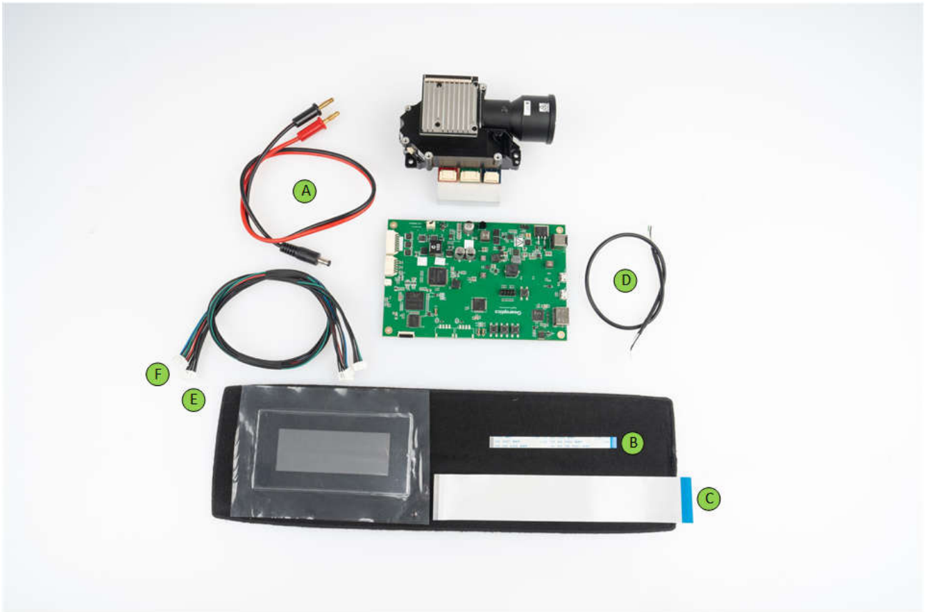
Figure 1-3. DLP4620SPGUQ1EVM Kitting List - Cable Designators
