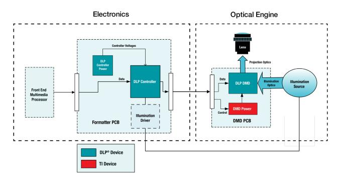
Figure 5. Typical DLP technology display system block diagram.
