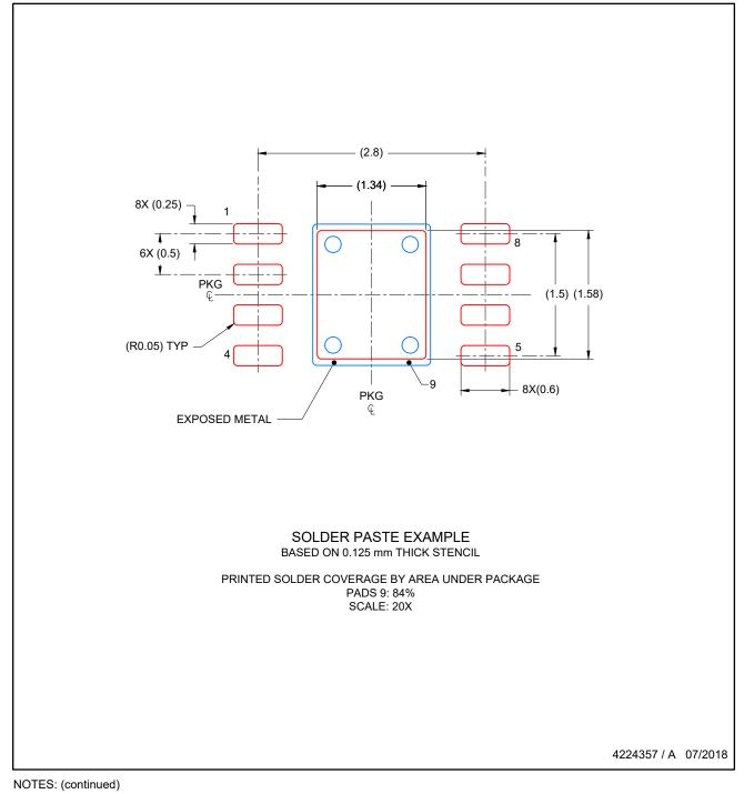
5. Laser cutting apertures with trapezoidal walls and rounded corners may offer better paste release. IPC-7525 may have alternate design recommendations..
