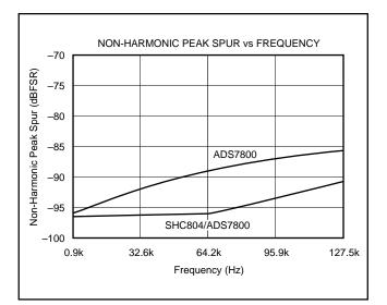
FIGURE 1. The Level of Non-Harmonic Spurious Signal Components is Improved by Using the Lower-Jitter Sampling Mechanism of the SHC804. Note that even without the SHC804, non-harmonic spurs are below –85dB up to the Nyquist frequency.
