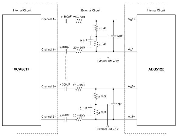
Figure 3. AC-Coupled Interface Between VCA8617 and ADS512x
