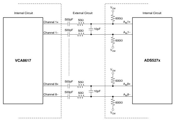
Figure 2. AC-Coupled Interface Between VCA8617 and ADS527x
