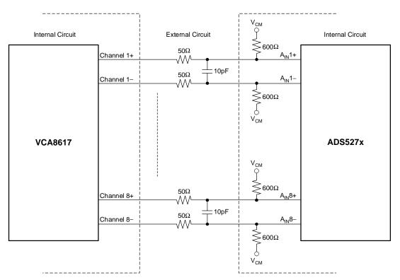
Figure 1. DC-Coupled Interface Between VCA8617 and ADS527x
