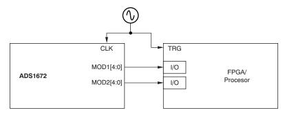
Figure 4. Hardware Connections
