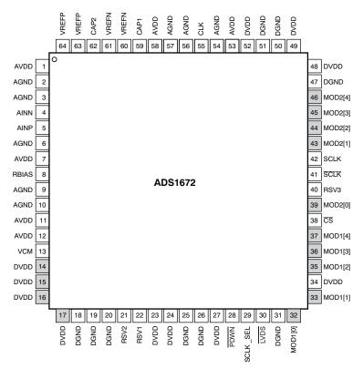
Figure 2. Bypass Mode Pinout
