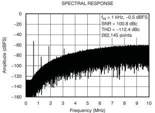
Figure 7. Spectral Response of Modulator Output at  $f_{IN} = 1 \text{ kHz}, -0.5 \text{ dbFS}$
