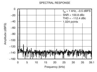
Figure 10. Enlarged View (8x) of FFT After 312.5 kHz Brick Wall Filter at  $f_{IN} = 1 \text{ kHz}, -0.5 \text{ dbFS}$
