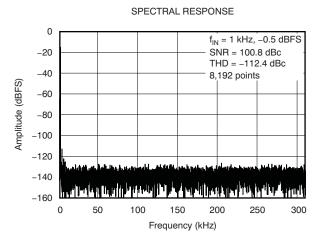
Figure 9. FFT After 312.5 kHz Brick Wall Filter at  $f_{IN} = 1 \text{ kHz}, -0.5 \text{ dbFS}$
