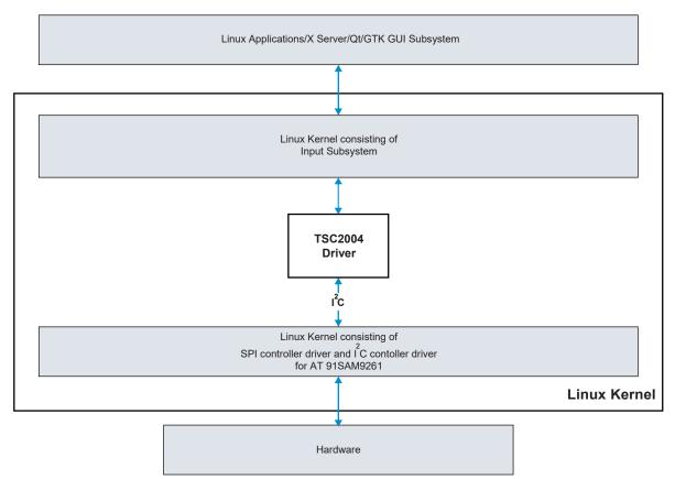
Figure 1. TSC2004 Linux Driver Architecture
