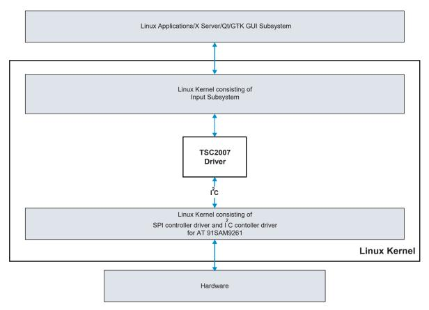
Figure 1. TSC2007 Linux Driver Architecture
