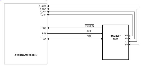
Figure 2. TSC2007 Connection Diagram
