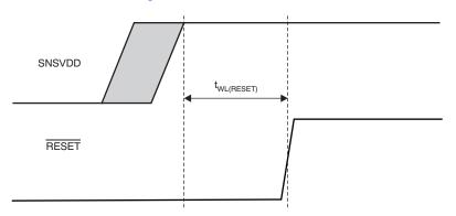
Figure 4. Recommended Hardware Reset During Power Cycle
