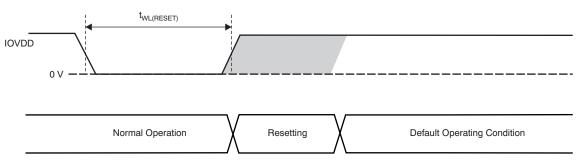
Figure 3. Hardware Reset Signal Specification
