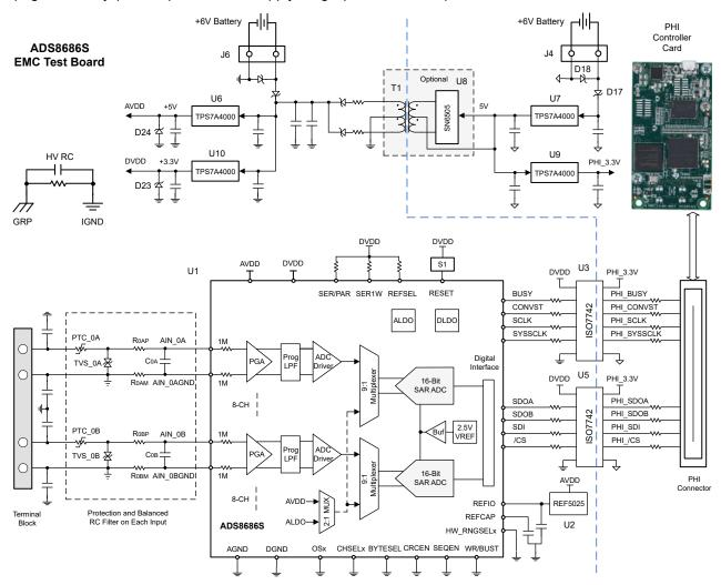
Figure 2-1. ADS8686S EMC Test Board Circuit
