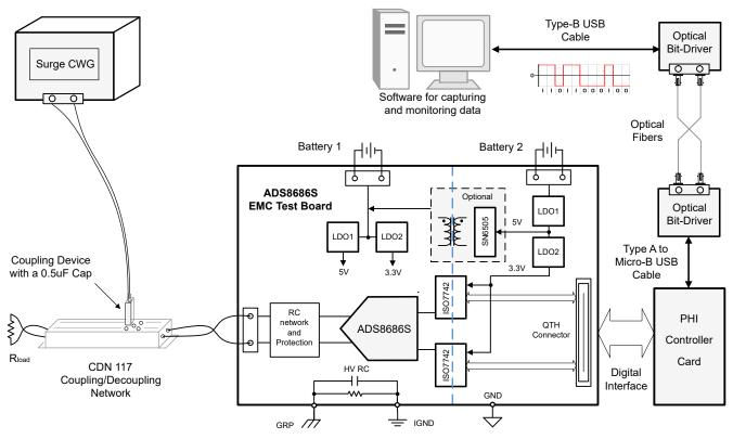
Figure 3-6. Diagram of Laboratory Setup for Surge Test
