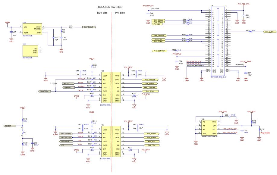
Figure 4-4. Schematic – Digital Isolation
