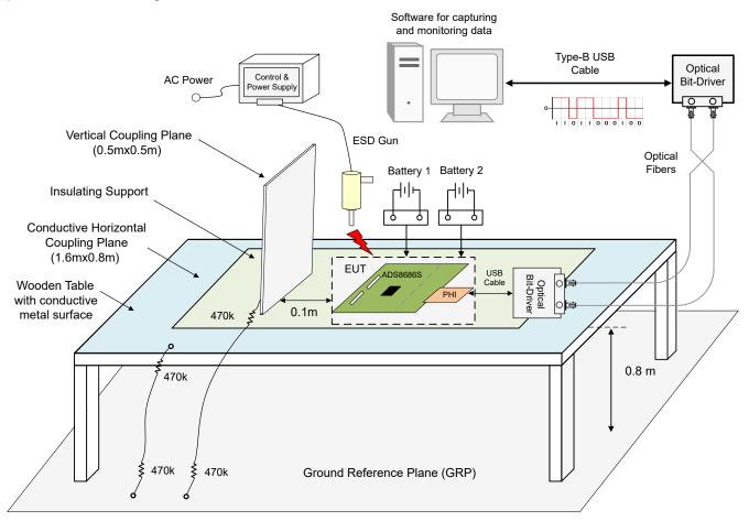
Figure 3-3. Diagram of Laboratory Setup for ESD Test
