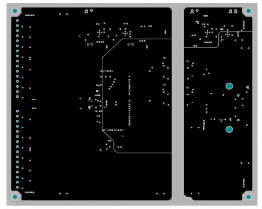
Figure 5-3. Layout – Inner Power Layer
