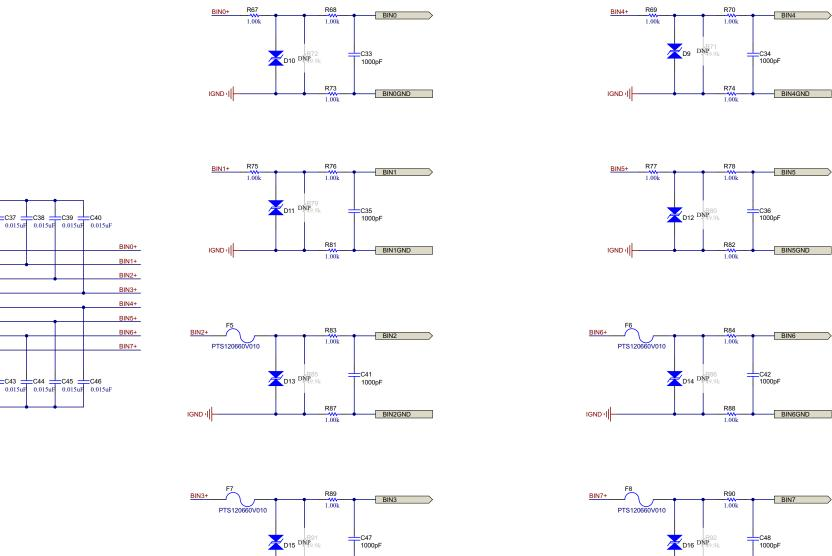
Figure 4-3. Schematic – Input of ADC - B
