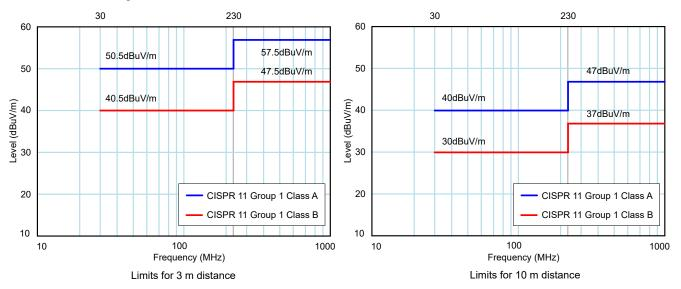
Figure 3-12. CISPR 11 Radiated Emission Limits for Class A and B Group 1 Equipment
