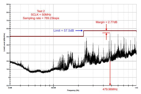
Figure 3-16. Test 2 - Measured Radiated Emission, Horizontal Antenna Polarization
