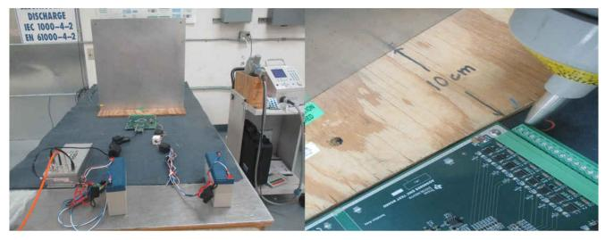
Figure 3-5. Photograph of Laboratory Setup for ESD Test
