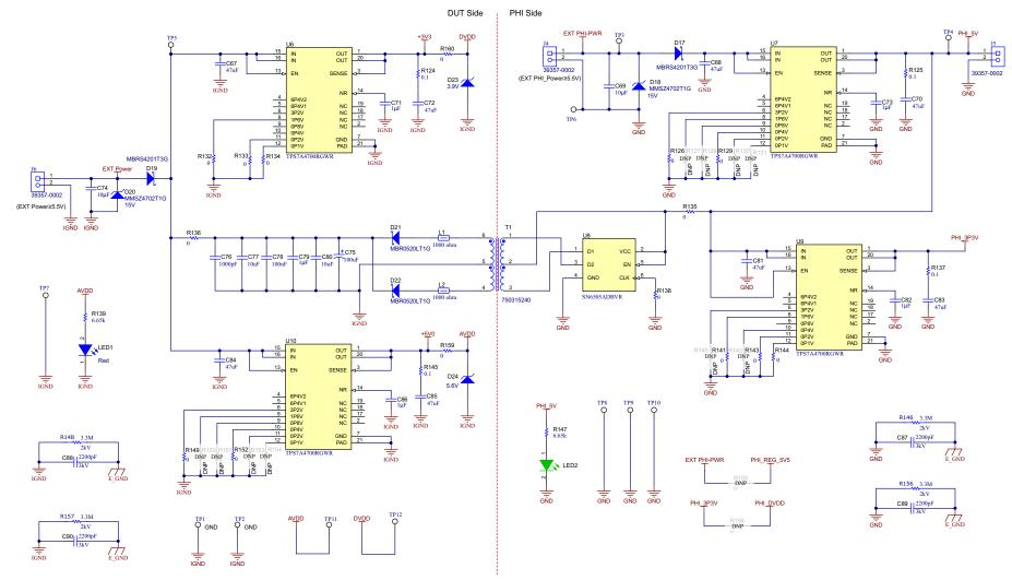
Figure 4-5. Schematic – Power Supply
