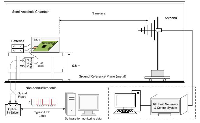
Figure 3-10. Diagram of Laboratory Setup for Radiated Immunity Test
