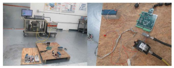
Figure 3-9. Photograph of Laboratory Setup for Conducted Immunity Test
