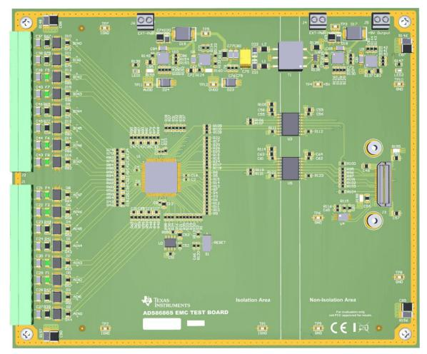
Figure 1-1. ADS8686S EMC Test Board
