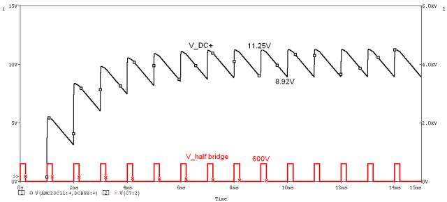
Figure 3-3. 1 kHz, 20% Duty Cycle Power Supply
