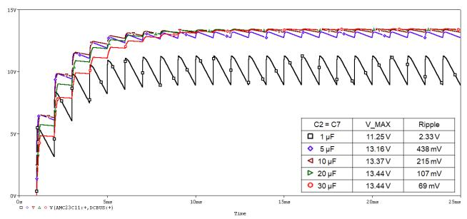
Figure 3-4. Increase Capacitor Value From 1  $\mu$ F to 30  $\mu$ F
