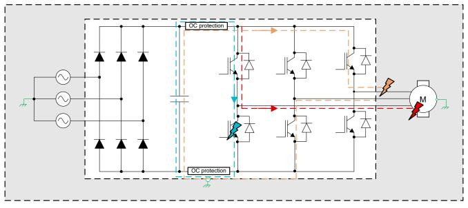
Figure 4-2. Add DC– Short-Circuit Protection
