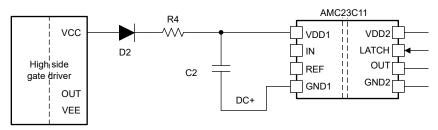
Figure 3-5. Low-Cost Power Supply Solution
