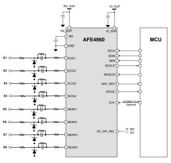
Figure 2. Wearable EEG System Using AFE4960
