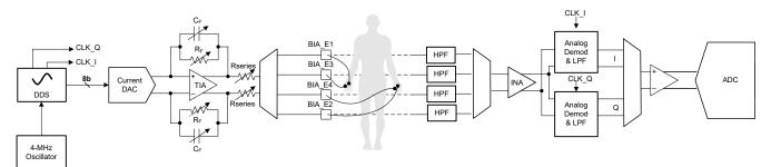
Figure 4. BIA Signal Chain in AFE4500
