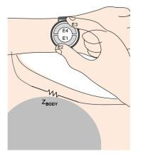
Figure 1. BIA Measurement on a Smartwatch
