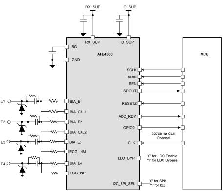
Figure 3. Reference Schematic Using AFE4500 for BCM on Wearables
