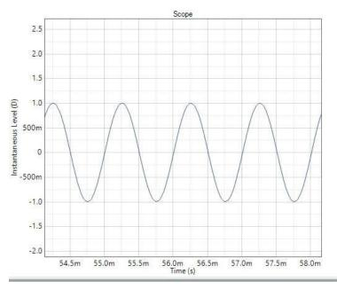
Figure 4-19. Digital Output Capture (Vin = 1 VRMS)
