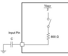
Figure 2-6. Quick Charge Circuit
