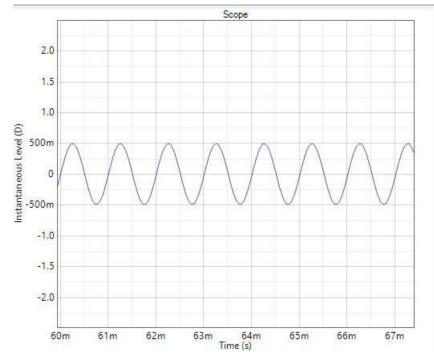
Figure 4-21. Digital Capture (Analog Differential Input of 1 Vrms)
