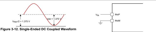
Figure 3-13. Single-Ended DC Coupled Circuit
