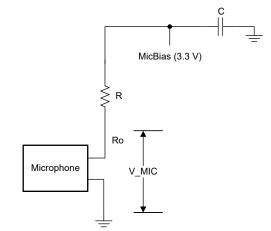
Figure 4-4. Single-Ended AC Coupled Condenser Microphone Test
