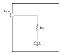
Figure 3-11. Equivalent Circuit of Input Pin
