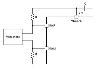
Figure 4-9. Circuit DC-Coupled Differential Microphone
