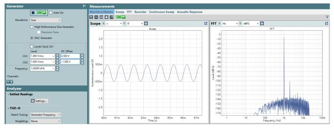
Figure 3-9. Digital Capture With Low-Pass Filter
