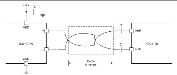
Figure 4-12. MEMS Microphone Connected Through Long Cable to ADC
