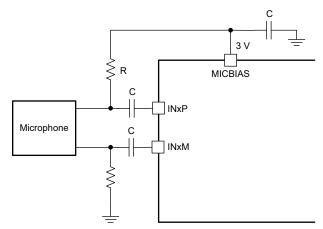
Figure 4-11. AC Coupled Differential Microphone Circuit
