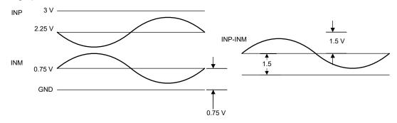
Figure 3-6. Input Pin Waveforms With Different Static DC Levels
