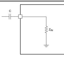
Figure 2-5. AC Equivalent Circuit of Input Pin
