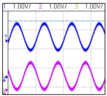
Figure 3-7. Waveforms at INxP and INxM Pins
