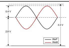
Figure 3-3. Biasing INxP and INxM at a Higher Voltage
