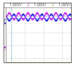
Figure 3-5. Input Pin Waveform 0.5-V Pk Signal on DC Bias of 2.5 V
