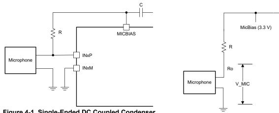
Figure 4-1. Single-Ended DC Coupled Condenser Microphone Circuit
