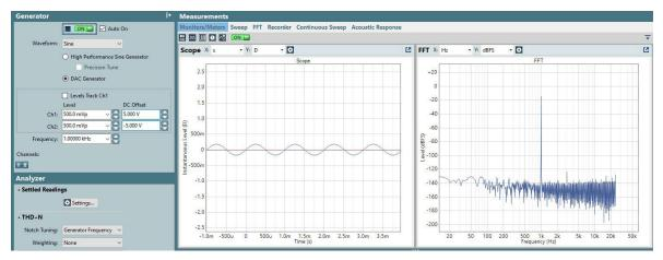
Figure 3-4. 0.5-V Pk Signal on DC Bias of 2.5-V-Input Pin Waveform and Digital Capture
