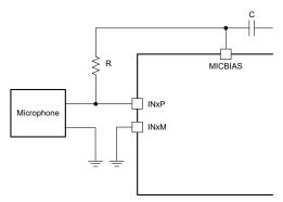
Figure 4-18. Single Ended DC Coupled Microphone Circuit
